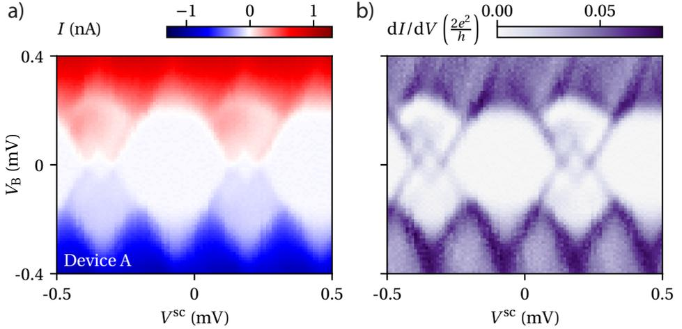
Figure 5.7: **Coulomb blockade measurements of the superconducting island in device A.** Left panel: current data, right panel: differential conductance obtained by taking the numerical derivative of the current data.
