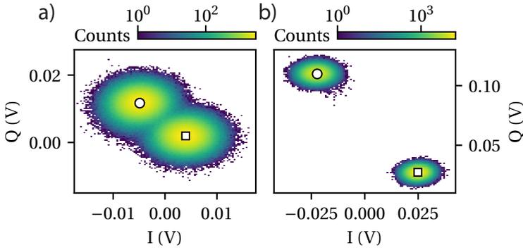
Figure 6.8: **Supplemental data for SNR measurements.** Histograms of the resonator response in the IQ plane with a pulse length of  $t_{\text{int}} = 1 \mu\text{s}$ , corresponding to the two regimes in Fig. 6.5. Both histograms contain measurements for Coulomb blockade (square marker) and on charge degeneracy (circle marker). **a)** Histogram for  $t_C = 4.5 \text{ GHz}$  and  $V_e = 5 \mu\text{V}$ . **b)** Histogram for  $t_C = 13 \text{ GHz}$  and  $V_e = 0.16 \text{ mV}$ .
