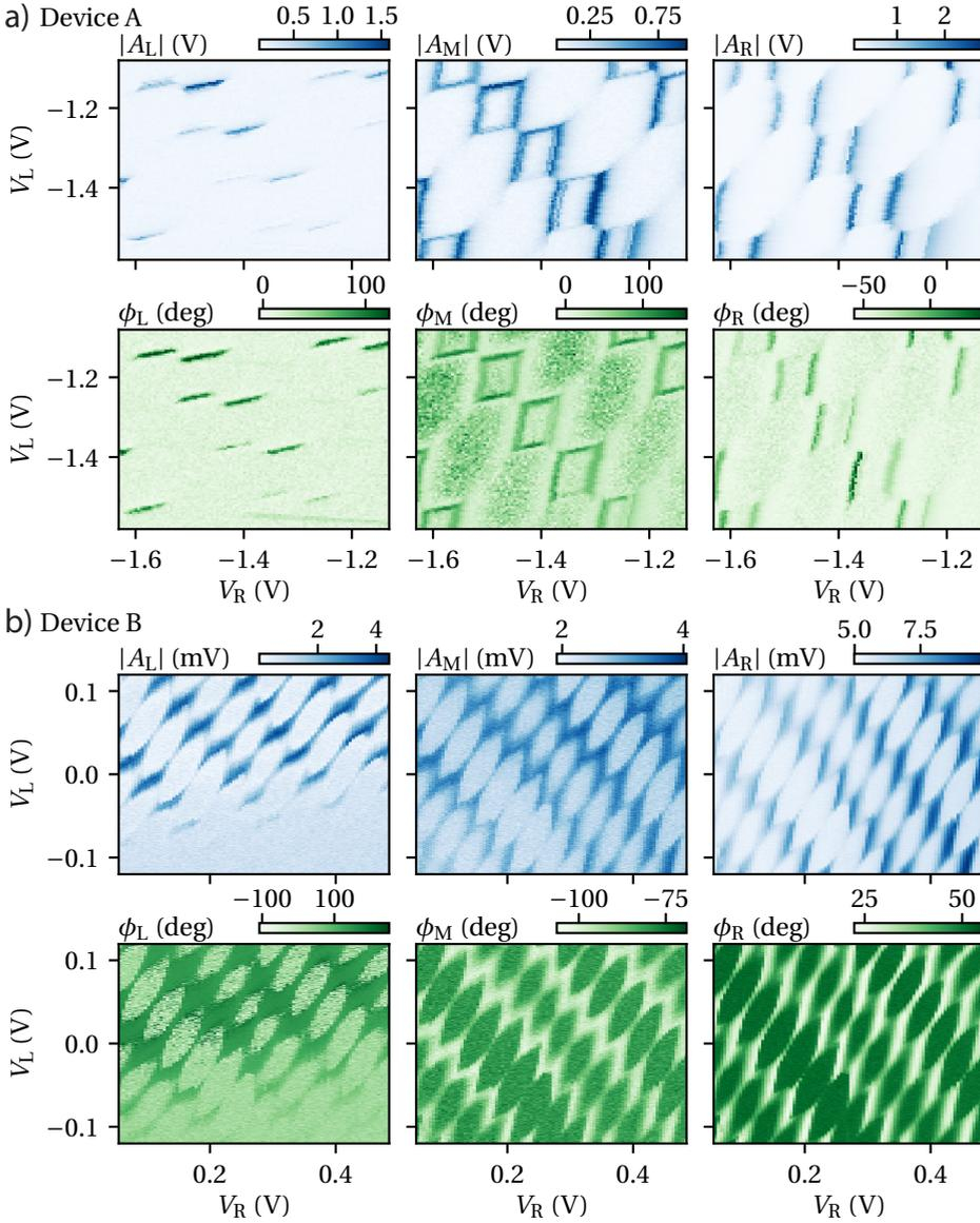
Figure 7.5: The individual resonator responses corresponding the two CSDs shown in Fig. 7.1c. Here,  $|A_i|$  and  $\phi_i = \arg(A_i)$  denote the amplitude and phase response of resonator  $i$ . **a)** Shows the response of device A while **b)** shows the response of device B.
