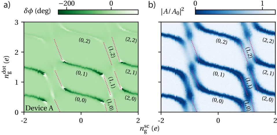
Figure 5.8: **Charge stability diagram measured with gate sensing via the plunger gate of the SC.** Left: phase, right: amplitude. The pink-dashed lines indicate, as guides to the eye, the SC-lead transitions.
