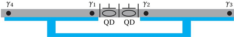
Figure 8.2: **Alternative geometry for the Majorana box qubit.** The advantage of this geometry is that it only needs a single, linear nanowire to realize. Figure adapted from Ref. [26]
