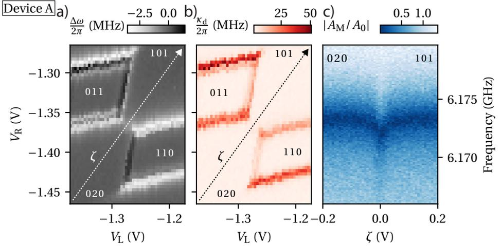
Figure 7.2: **Middle resonator response in the floating triple dot regime.** a), b) The resonance frequency,  $\Delta\omega$ , and linewidth,  $\kappa_d$  of the middle resonator. The values are from the frequency response of the middle resonator for every point in the charge stability diagram. c) Frequency response of the middle resonator across the Cooper pair splitting transition. The gate voltage,  $\zeta = V_L + V_R - V_{\text{offset}}$  is defined in a) and b) by the dashed arrow.
