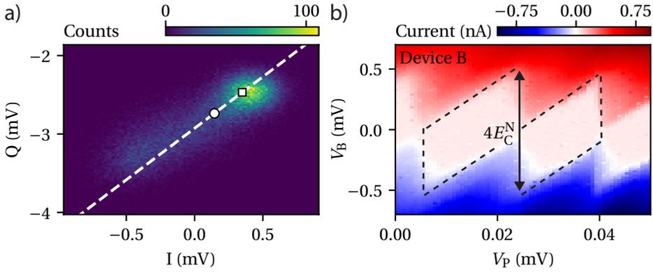
Figure 7.7: **a)** Histogram of the IQ response of the middle resonator, corresponding to the middle panel in Fig. 7.5b. The square marker denotes the most occurring IQ response which we associate with Coulomb blockade while the circle marker denotes the average IQ response. These markers define the dashed line which is used to project the complex-valued data. **b)** Current measurement of Coulomb diamonds for QD P in device B. From the bias axis, we infer  $E_C^N = 250\mu\text{eV}$ .
