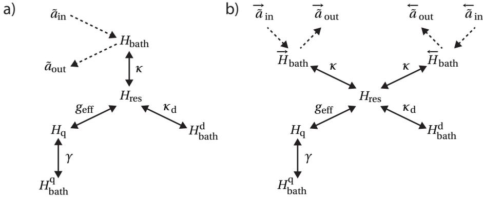
Figure 2.6: Schematic representation of the Hamiltonian describing the resonator response **a)** in reflection and **b)** in the hanger geometry. The bath Hamiltonians have been given different indices to signify they represent distinct environmental modes. Solid arrows represent coupling between different parts of the Hamiltonian, while the dashed arrows represent the relevant input and output modes.
