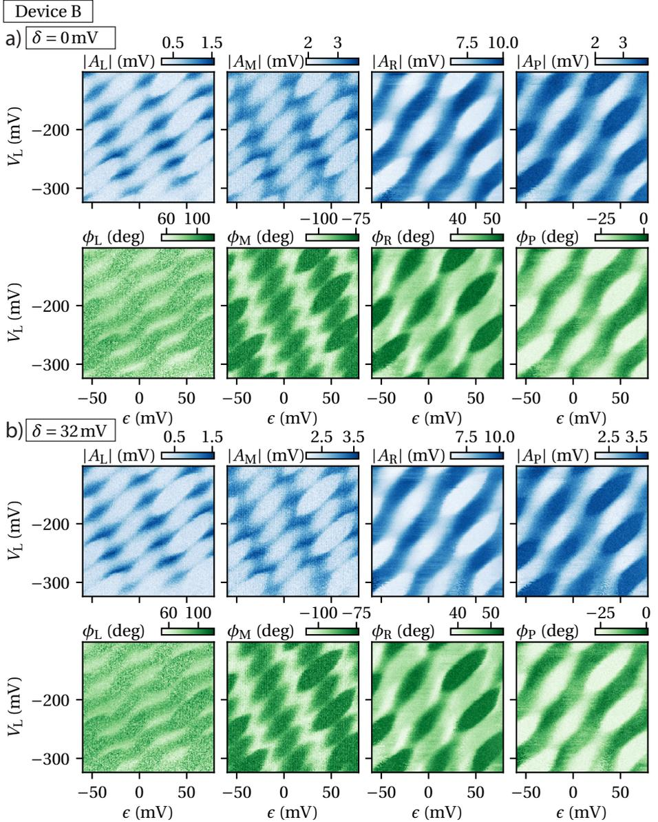
Figure 7.6: The individual resonator responses corresponding the CSDs shown in Fig. 7.3b. Here,  $|A_i|$  and  $\phi_i = \arg(A_i)$  denote the amplitude and phase response of resonator  $i$ . Even though the response of resonator P is not included in the colormap (see Fig. 7.3e), it is added here for completeness. a) A slice from the CSD taken at a detuning of  $\delta = 0 \text{ mV}$ . b) A different slice from the same CSD taken at a detuning of  $\delta = 32 \text{ mV}$ .
