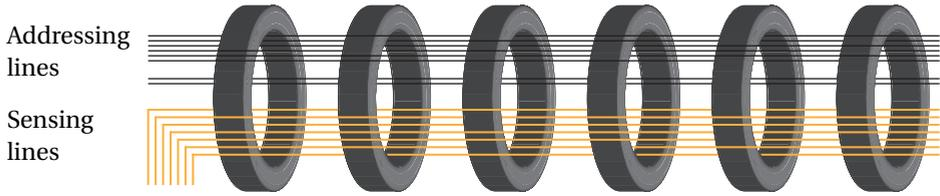
Figure 1.1: **Topological protection of classical computer memory.** A schematic representation of Core rope memory, adapted from Ref. [13]. The sensing lines, shown in yellow, encode a 0 or 1 by either bypassing or threading through the individual core.
