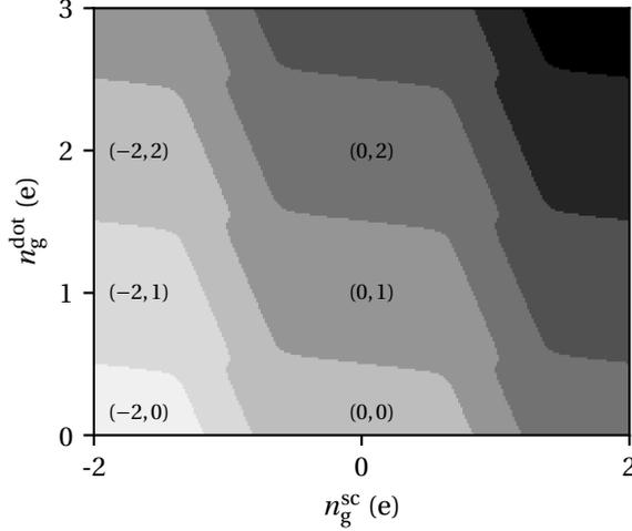
Figure 5.9: **Simulation of the charge stability diagram of Fig 5.2 of the main text.** The gray scale indicates the sum of the charge in the hybrid double dot.
