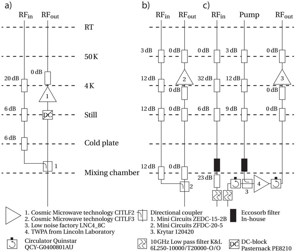
Figure 3.5: **a)** Schematic of the UHF reflectometry setup in the Leiden Cryogenics cryostat. **b), c).** Schematic of the UHF and SHF measurement setup in the Bluefors cryostat, respectively.
