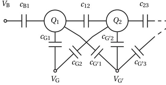
Figure 2.1: Schematic of the capacitance network corresponding to a multi quantum dot system. The quantum dots 1 and 2 are denoted by large circles and form the charge nodes in the system. The smaller circles represent the voltage nodes and tune the electrostatic environment of the quantum dots. The bias node and two gate nodes are labeled by B, G, and G' respectively.
