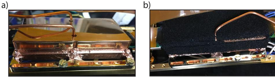
Figure 3.4: **a)** Copper casing enclosing the sample. Holes for the RF lines are not sealed yet. **b)** Eccosorb foam placed around the copper box to absorb any stray radiation in the puck.
