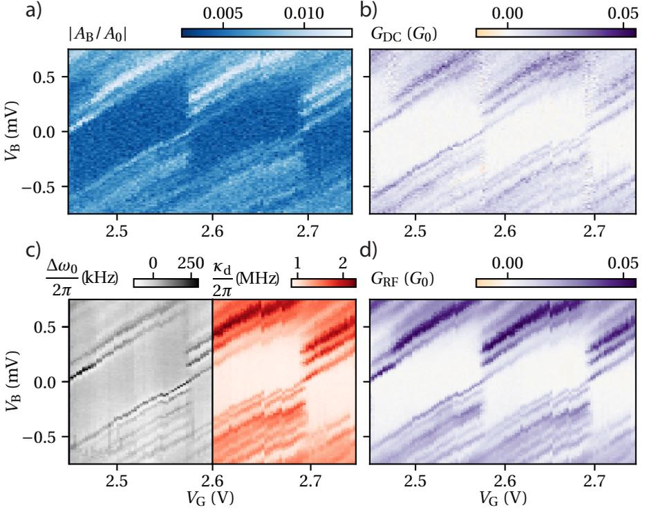
Figure 6.3: **Coulomb blockade diamonds measured in a single quantum dot.** **a)** Single-frequency response of the resonator. **b)**  $G_{DC}$  measurements obtained with standard lock-in techniques. **c)** Frequency shift  $\Delta f$  and resonator decay rate  $\kappa_d$  extracted from frequency traces. **d)** Conductance  $G_{RF}$  extracted from resonator data in **c)**.
