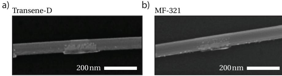
Figure 3.2: a) Result of etching with Transene-D. b) Etching with MF-321 leaves clear residu on the etched part of the nanowire which is assumed to be  $\text{AlO}_x$ .
