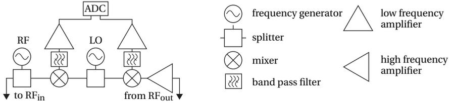
Figure 3.6: Schematic of the room temperature demodulation circuitry. The exact implementation differs slightly for the different experiments in this thesis. For clarity, the repeated circuitry for multiplexing is not shown.
