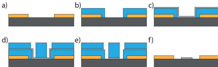
Figure 3.3: Schematic illustration of the fabrication of a local gate dielectric. **a)** Substrate in dark gray with resonators in orange. **b)** A liftoff resist mask (blue) is patterned. **c)** The dielectric is deposited (light gray). **d)** A second resist mask (blue) is put on top and patterned. **e)** The exposed dielectric is etched. **f)** All resist is removed from the sample.
