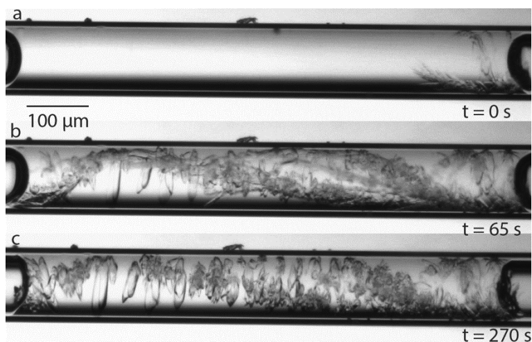
Figure 3.4: Crystallization of 1 \text{ mol kg}^{-1} sodium sulfate solution mixed with 0.051 \text{ mol kg}^{-1} borax in a glass capillary at the start (a) and after 65 s (b) and 270 s (c). Both phase III and phase V anhydrous crystals form simultaneously (a). At the end of the shown sequence (c), all the needles (phase III) have dissolved. The crystal habit of phase V is altered with respect to that observed in the absence of borax (compared to Figure 3c).
