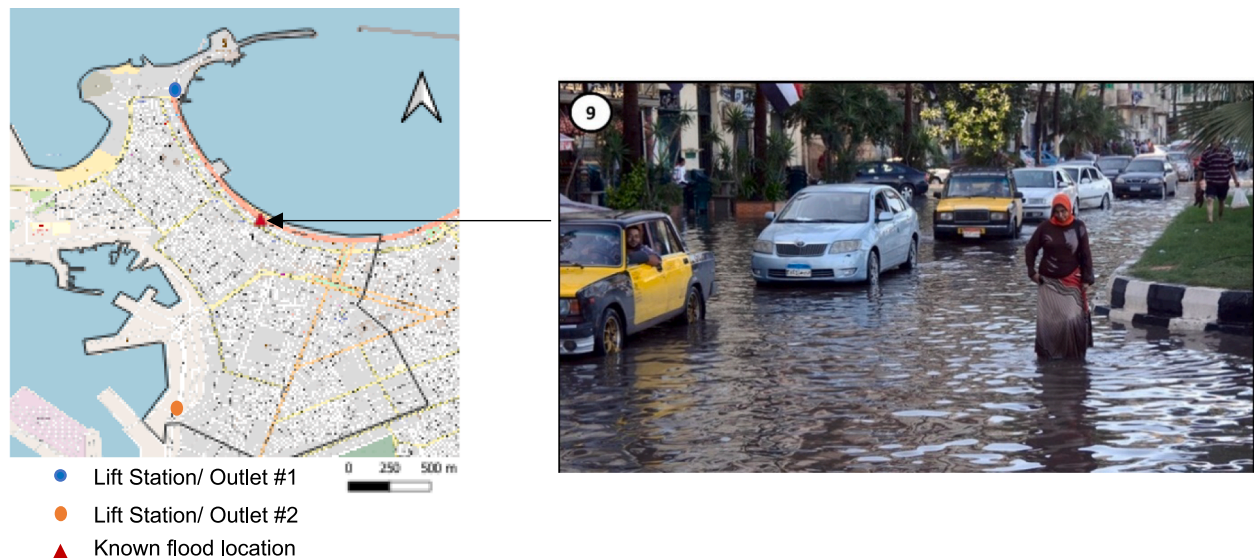
Fig. 16. Known flooding locations in El Gomork along the Corniche Road in Alexandria. On October 25, 2015, this location experienced flooding depths \sim 0.15 – 0.3 m.
