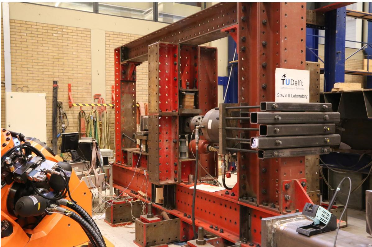
Figure 5.1: Specimen 2E1 in test set-up
