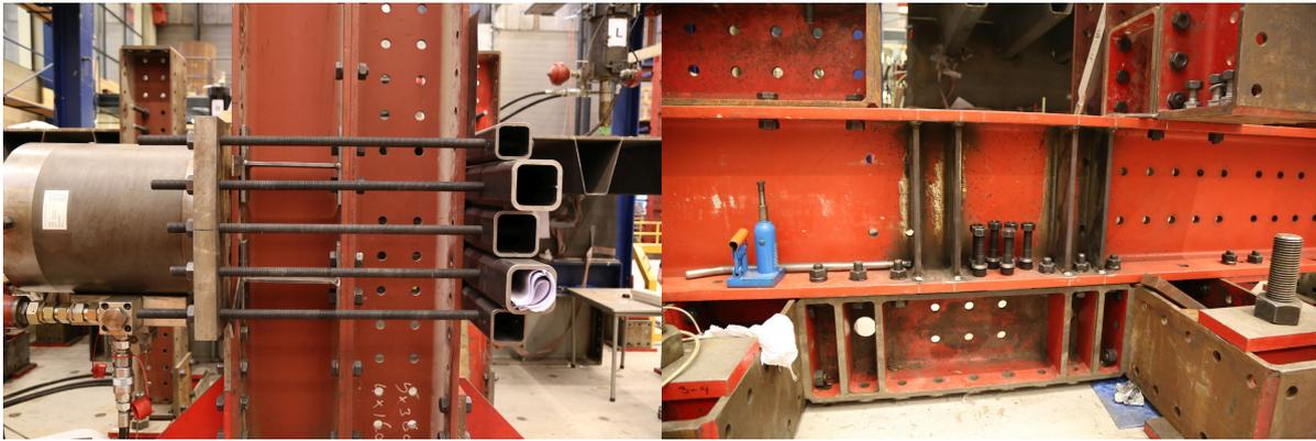
Figure 5.7: Specimen clamp and jack mount
