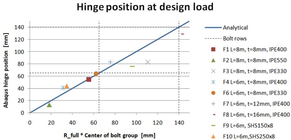
Figure 9.14: Abaqus results for the hinge position and analytical results based on R
