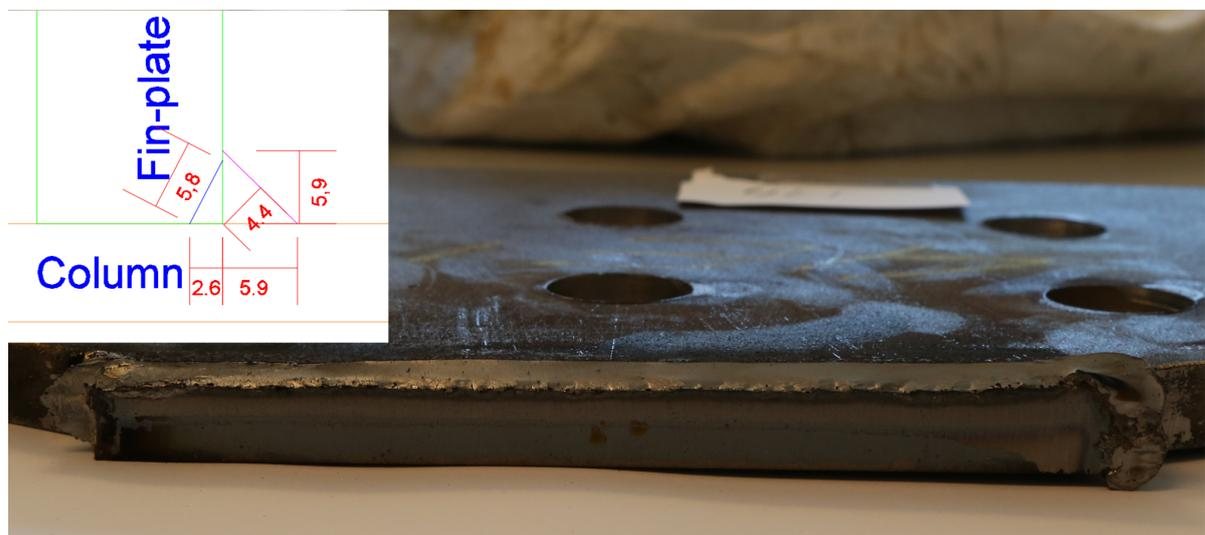
Figure 5.19: 4E1 failure plane after testing
