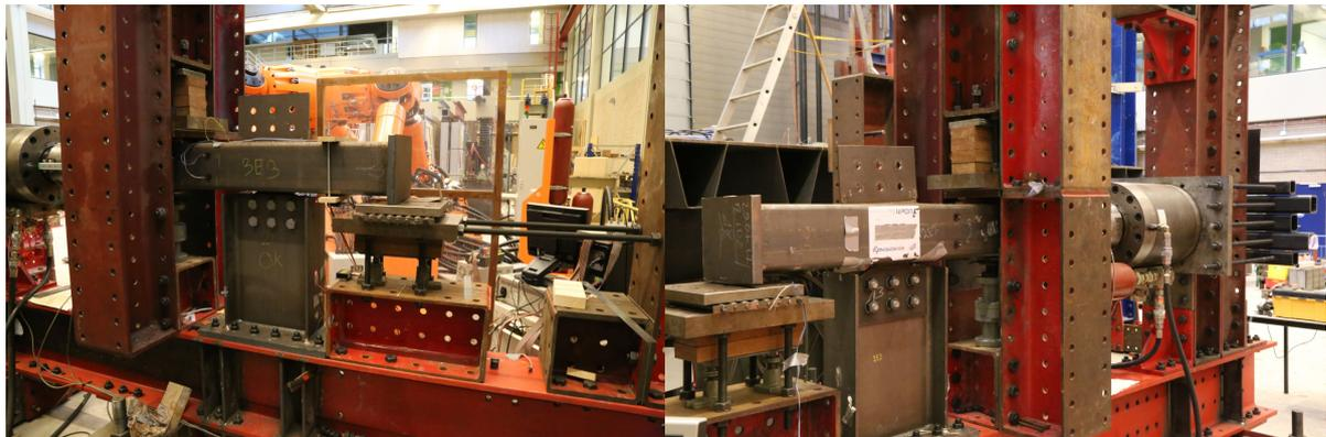
Figure 5.6: Roller supports
