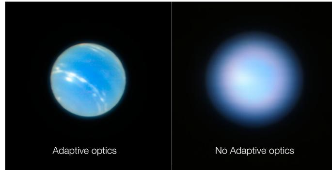
**Figure 2-1:** Neptune with- and without Adaptive Optics. [1]
