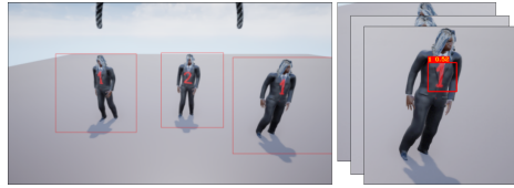
Figure 3.4: Pedestrian models, as seen from the drone’s perspective in the realistic environment. Each pedestrian is tracked using AirSim’s API. Its class is represented by a red number in the front, classified using YoloV3.
