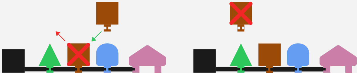
Figure 7. Daisy chain (line) modular architecture allows for easy replacement of modules along a linear track without affecting surrounding modules.
