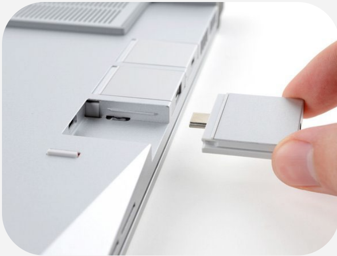
Figure 14. The expansion card mechanism on a Framework laptop
