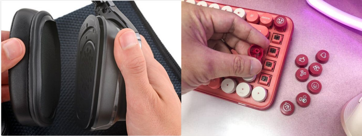
Figure 10. Replaceable earcups on the Logitech G935 headphones.
