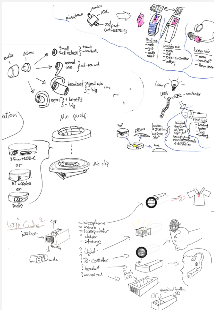
Figure 118. Ideas generated by stripping PC peripherals to their bare bones, and then using modules to build them back up.
