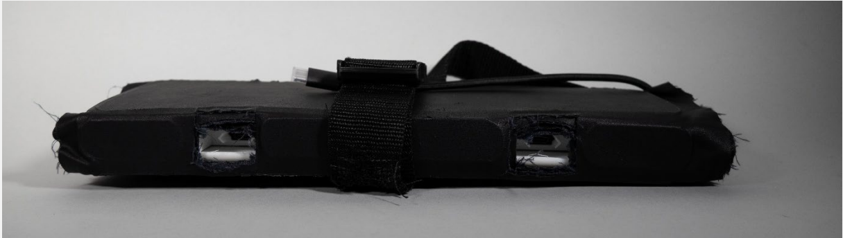
Figure 70. Back view of the rolled-up hub, displaying the two ports that are still accessible in this configuration.
