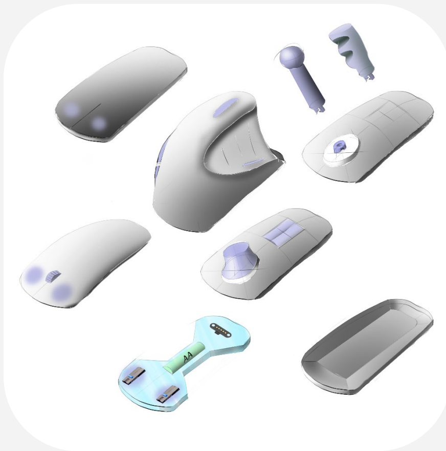
Figure 41. The barebones mouse (bottom left, blue) together with all types of modules that can be attached to the base mouse.
