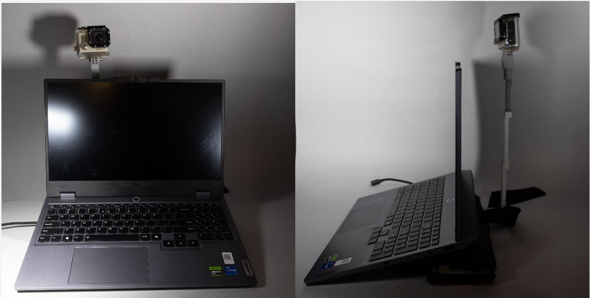
Figure 72. Front and side view displaying the hubs capability to build up modules in 3D space, in this case a stand for a GoPro, to be used as a webcam.
