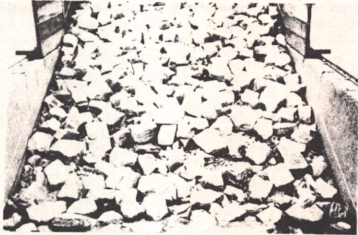
Rock overlay in large wave tank at the Coastal Engineering Research Center (CERC).
