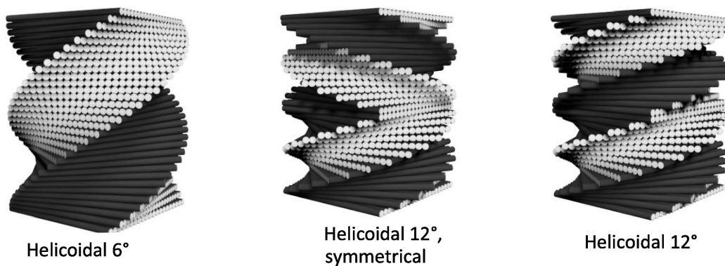
Figure 2.12: Various helicoidal layup configurations [104]
