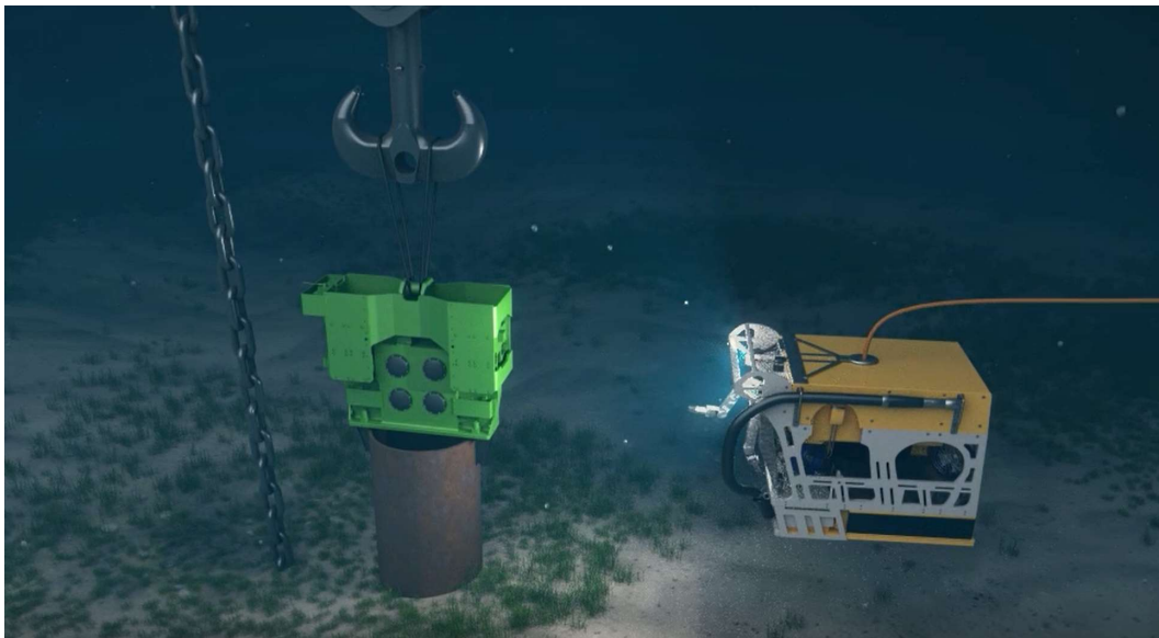
Figure 7: ROV inspecting pile driving
