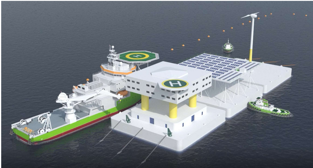
Figure 11: OCV disconnecting the mooring lines while tugboats are ready for towage
