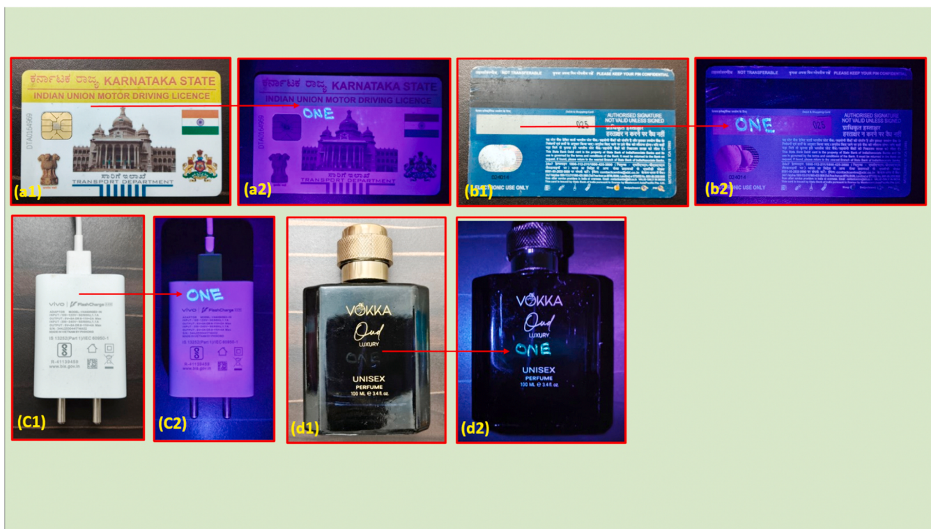
Fig. 20. Anti-counterfeiting labels with \text{Dy}_2\text{O}_3:\text{Er}^{3+} (9 mol%) nanoparticles passivated with 9 wt% PVP ink under visible light (a1-d1) and (a2-d2) 365 nm UV light.
