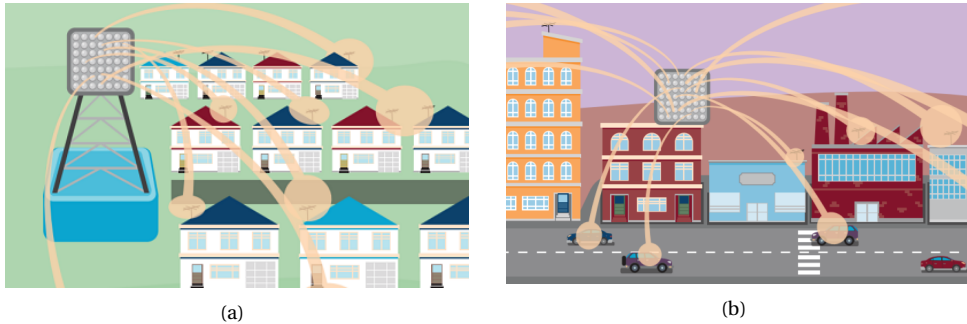
Figure 1.4: 5G mm-wave base station deployment scenarios [16]: (a) fixed wireless access in suburban environments, (b) fixed and mobile deployment in dense urban environments.
