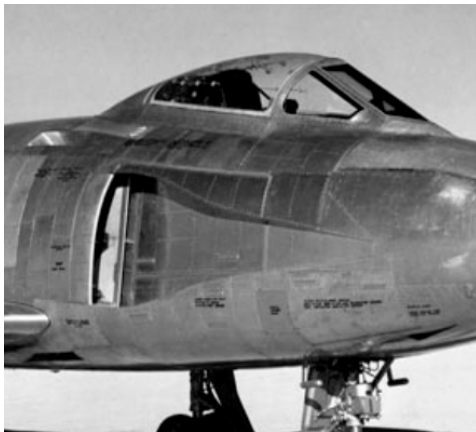
Figure B.10: A NACA intake used as primary intake on the YF-93. [82]
