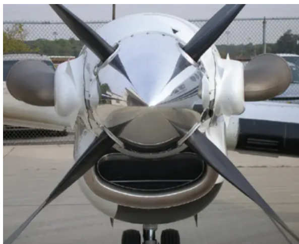
Figure B.4: Example of a scoop intake on a turboprop engine. [78]
