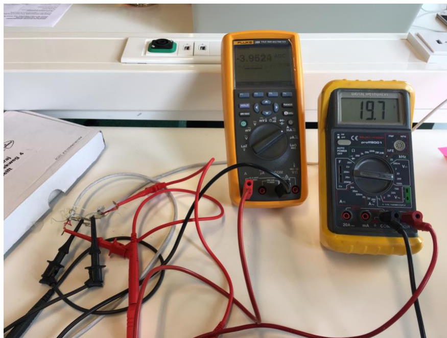
Figure A.1: Initial setup used for measuring AC/DC and DC/DC converter output
