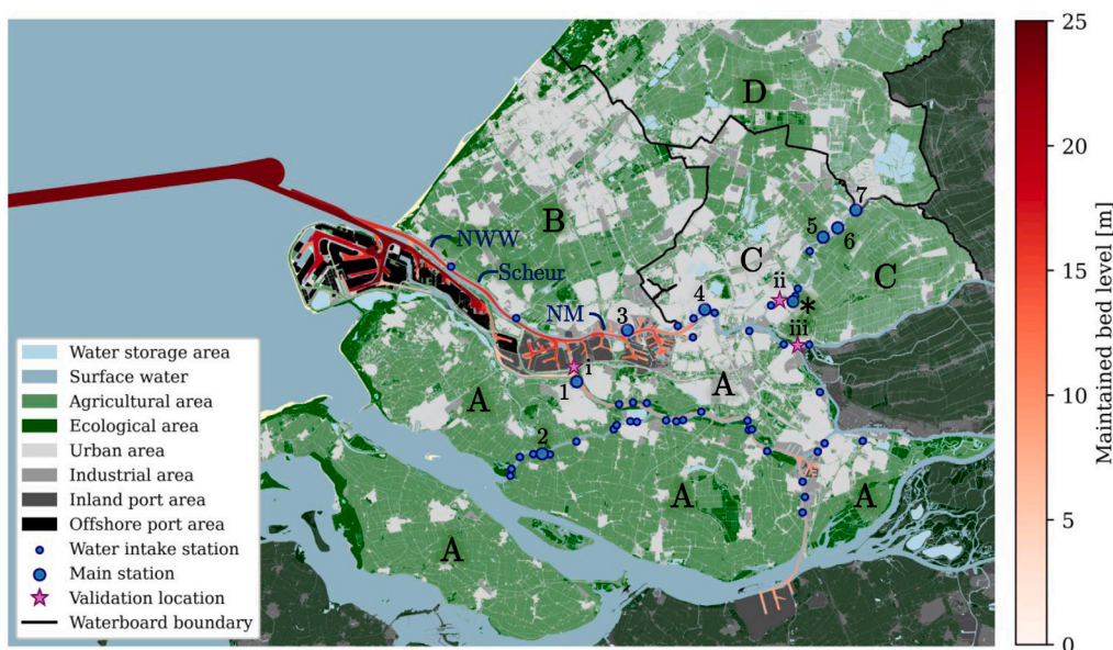
Fig. 2. Overview of the land-based and water-based functions in the RMD, including the design of MBL of the PoR, and the water boards (A – D) and their water intake stations (1 – 7). The asterisk * marks the location of representative hydrodynamic data for water intake stations 5, 6, and 7 (upstream of the Hollandsche IJssel river). The locations of measurement data are: (i) Spijkenisse-brug, (ii) Krimpen a/d IJssel, and (iii) Kinderdijk.
