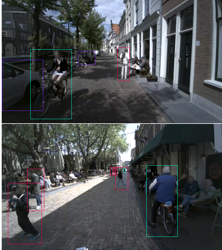
Figure 4.2: Example frame annotations following defined labelling rules. Only traffic participants clearly within the cyclist’s field of view are labelled.
