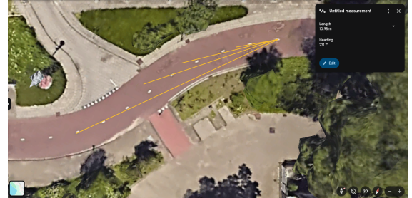
(b) Top-down reference with ground-truth spacings. The orange lines represent the line distances between the cyclist and observed tracks in the image on the left.
