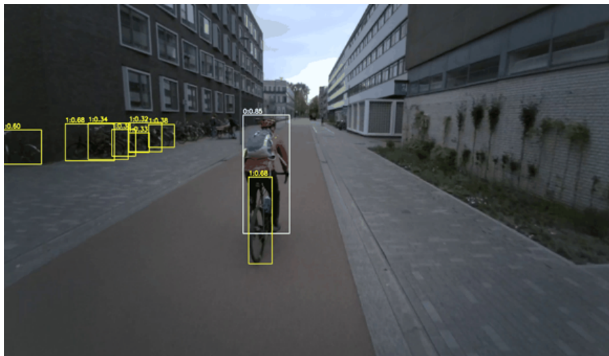
Figure 4.1: Example YOLO11m output on single frame, in yellow are the bicycle detections, white is the person class, class number and confidence scores are given on top of the detection boxes.
