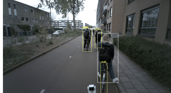
Figure A.5: Merge working only for 2/3 of the detected objects fully in view
