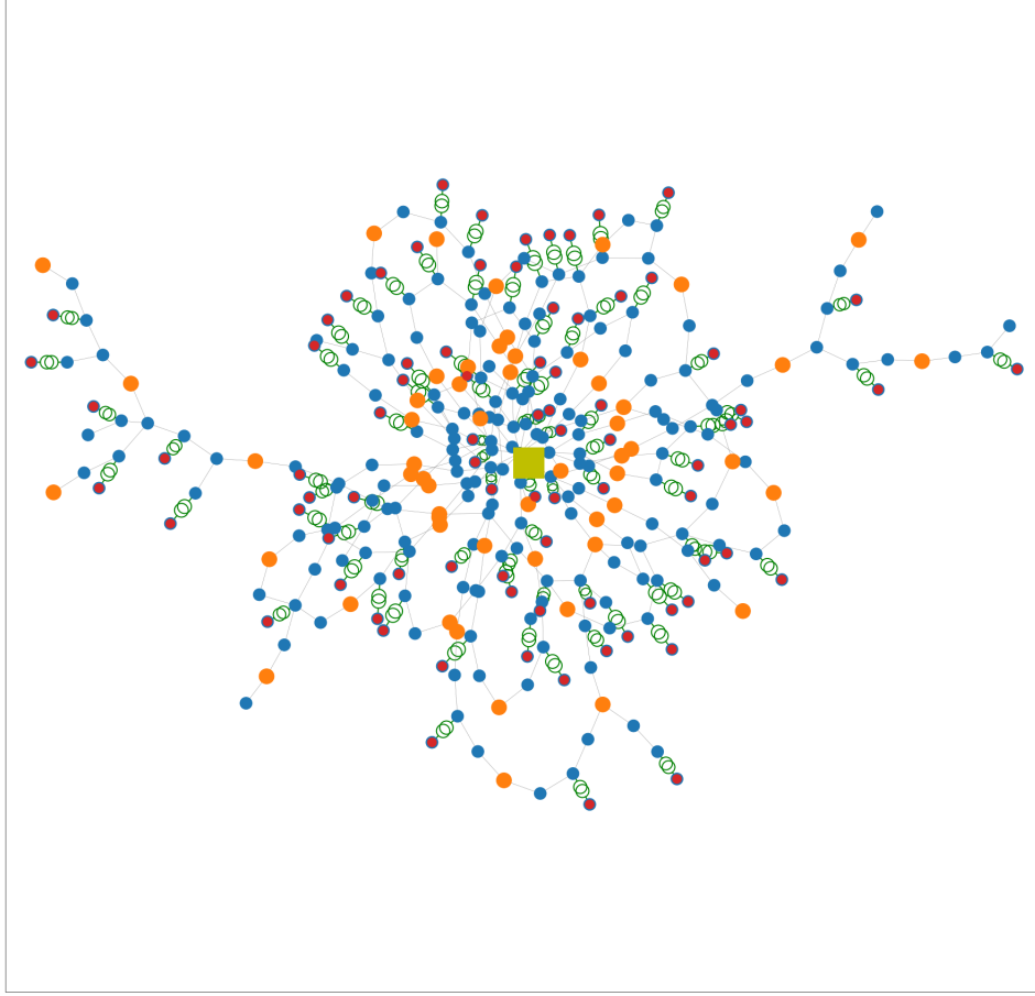
Figure 5.1: Placement of meters: Metered MV nodes are represented in orange and metered LV nodes are represented in red
