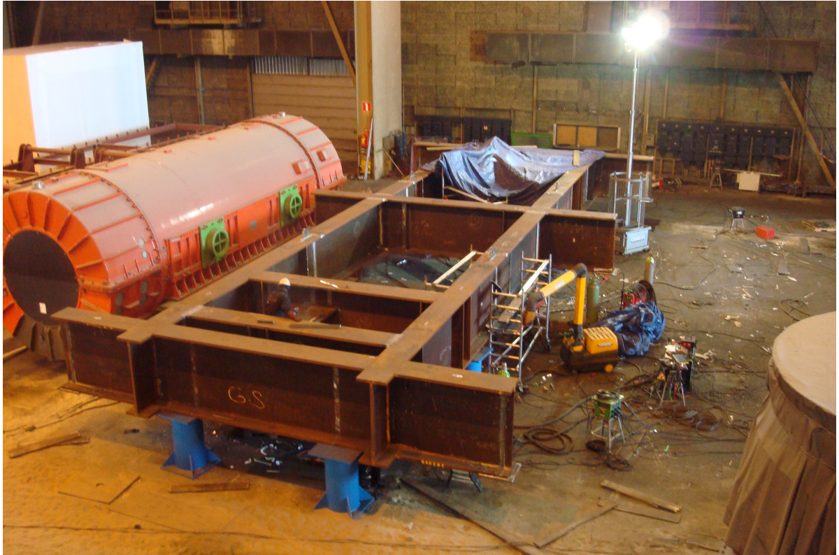
Figure 2.8: Topside grillage prefabrication – WindMW Meerwind Project (SHL)
