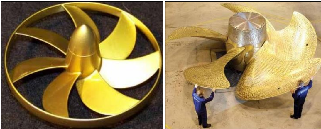
Figure 1: (left) Submarine propeller [1], (right) Adjustable, bolted propeller from the Queen Elizabeth class aircraft carrier [1].
