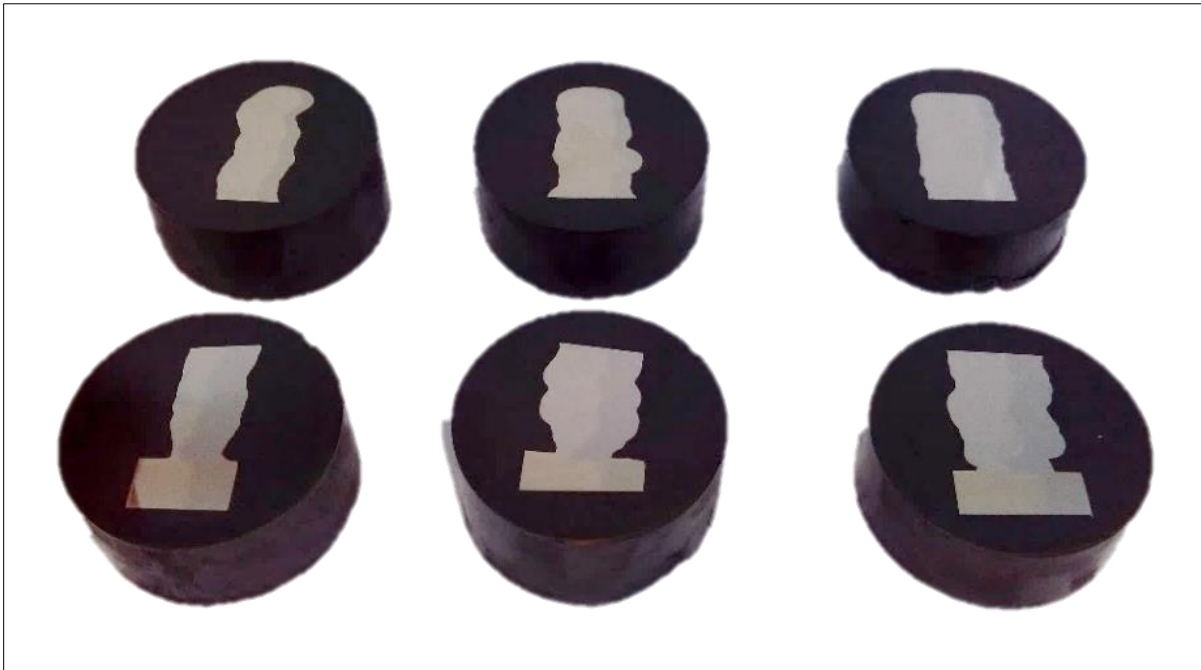
Figure 32: Mounted specimens with conductive phenolic resin, ready for observation in optical microscope and scanning electron microscopy (SEM). (left) Block A1, (middle) Block B1, (right) Block C1.
