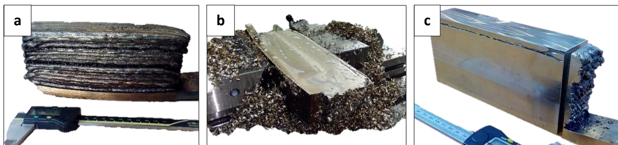
Figure 31: Pictures of the manufacturing process of the block produced at RAMLAB. (a) The as deposited block. (b) The block during milling. (c) The block after milling, ready for further machining, in order to produce tensile and Charpy specimens.
