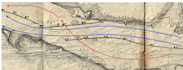
Figure 6.3: Secondary flow line (red) and primary flow line (blue) in point 2 (Own work)
