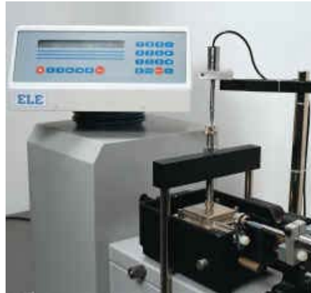
Figure 7.1 Set-up for the direct shear test
