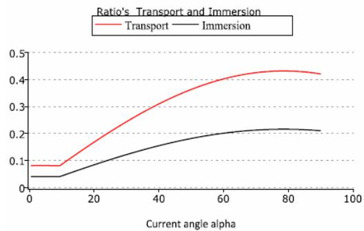
Figure 63  $H/B_{eff}$  ratio during transport and immersion
