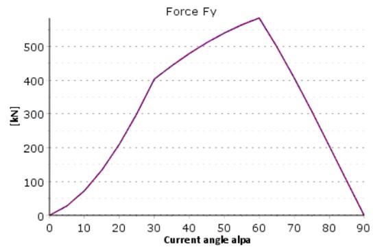
Figure 70 Force  $F_y$  as a function of the current angle  $\alpha$
