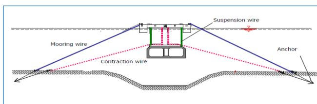
Figure 13 Tunnel element during the immersion (Wim Janssen, 2012)
