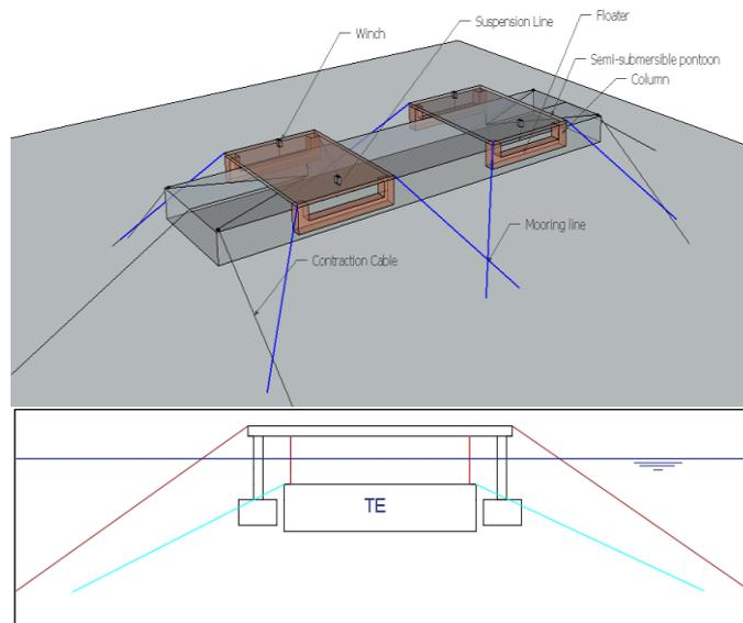
Figure 42 Semisubmersible pontoon
