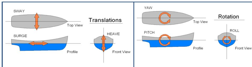
Figure 51 six degrees of freedom of a floating structure
