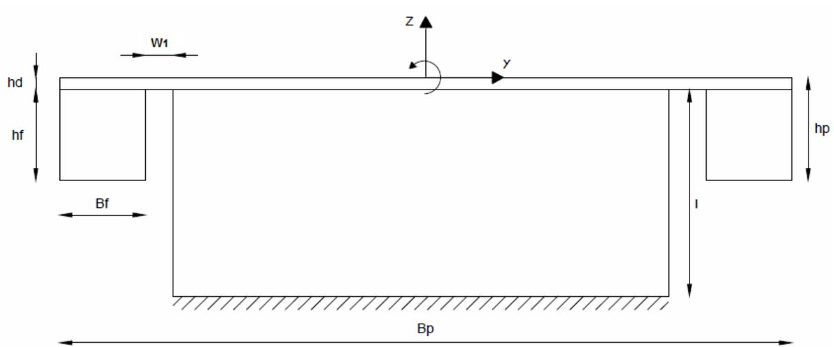
Figure 96 Modelled pontoon configuration during immersion
