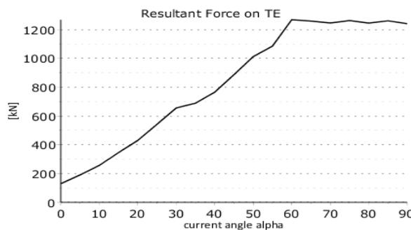
Figure 73 Resultant force  $F_R$  for 1 m/s flow velocity
