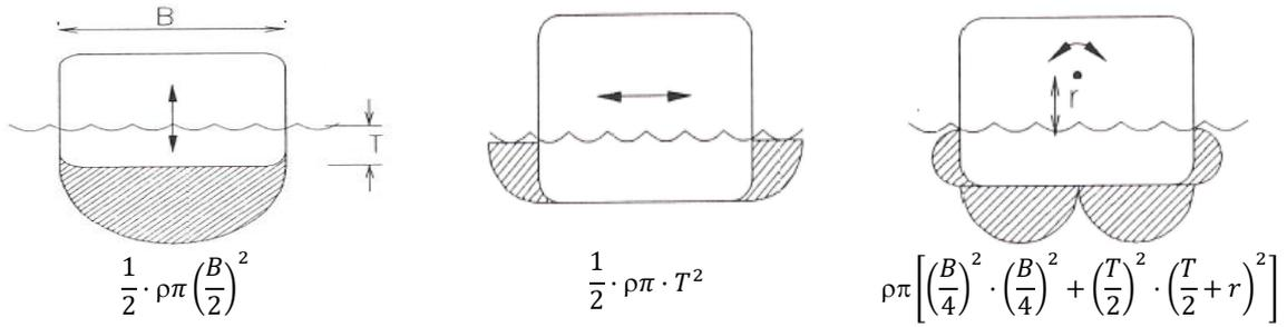
Figure 123 Estimate of added mass for water piercing parts (from Baltrop, 1998).
