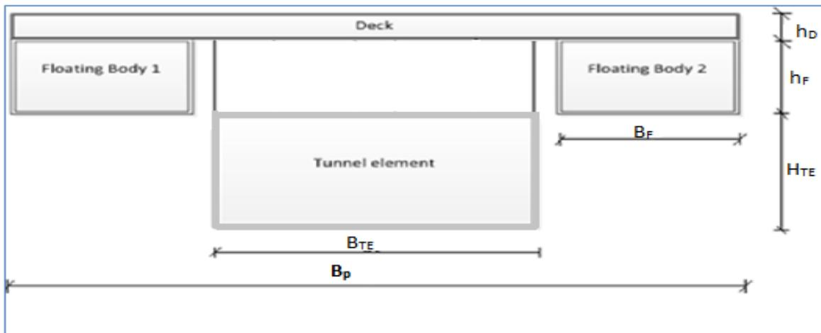
Figure 97 pontoon configuration during immersion with stationary tunnel element (drawing in not on scale)
