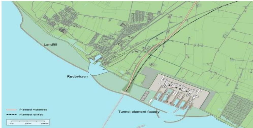
Figure 3 Tunnel production factory at east site of the Rødbyhavn (Femern A/S, 2013)
