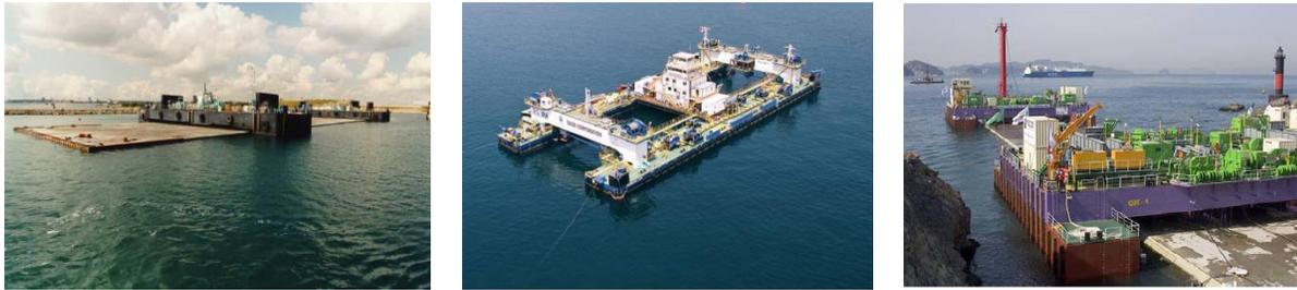
**Figure 5** different immersion pontoon types used in the projects (Oresund Fixed Link, Bosphorus Fixed Link and the Busan Geoje Fixed Link) [ (CAPITA SYMOND), (TAISEI Corporation , 2014), (Hans Cozijn and Jin Wook Heo, 2009) ]
