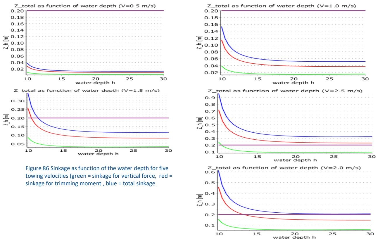
Figure 86 Sinkage as function of the water depth for five towing velocities (green = sinkage for vertical force, red = sinkage for trimming moment, blue = total sinkage)
