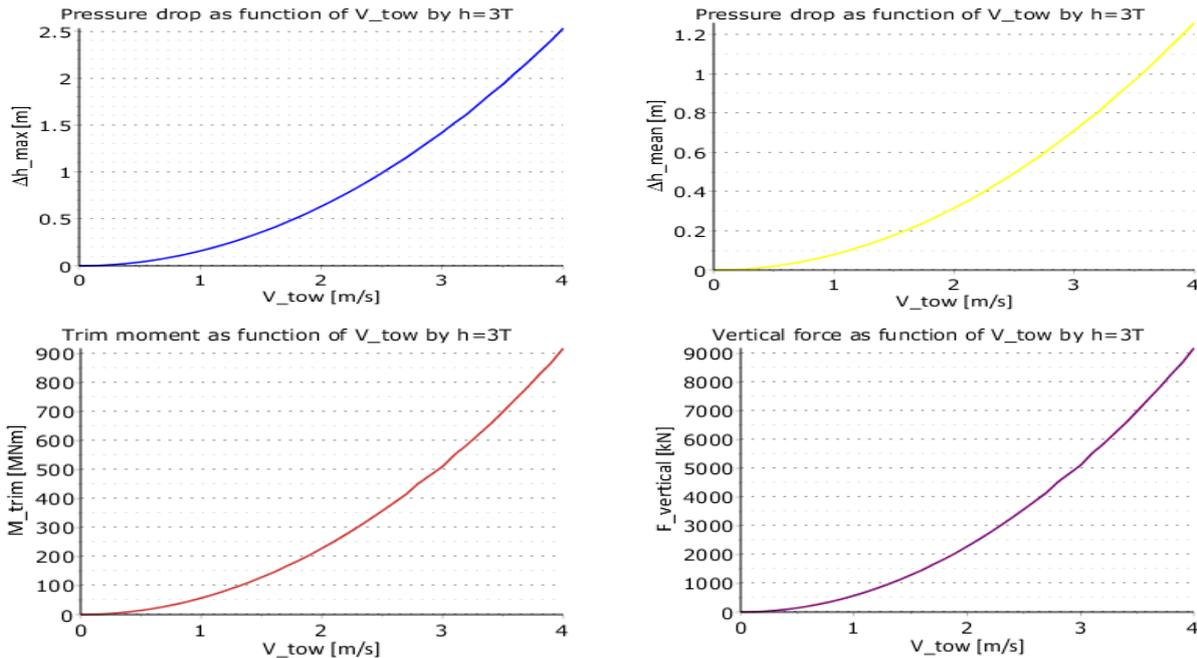
Figure 81 Pressure drop and the associated force as function of flow velocity
