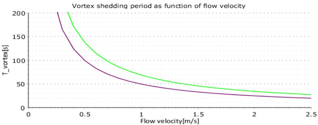
Figure 92 Vortex shedding period as function of flow velocity
