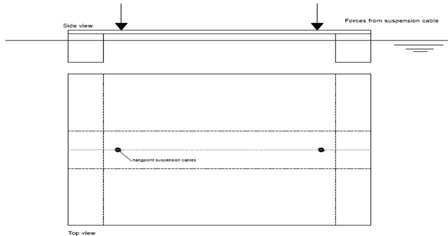
Figure 46 Principle of: working force from suspension cables on pontoon
