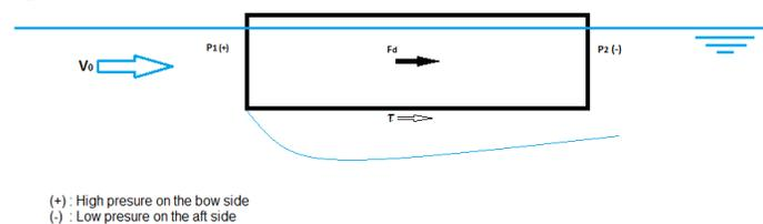
Figure 22 Principle of current force on TE during transport
