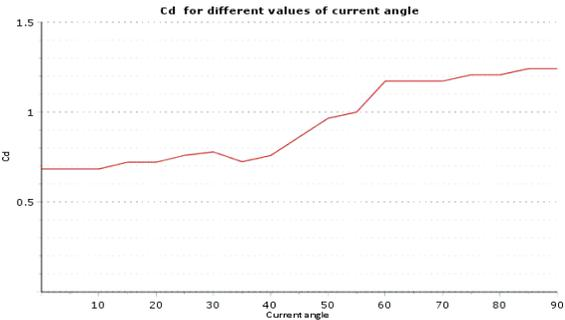
Figure 65 Drag coefficient for different current angles
