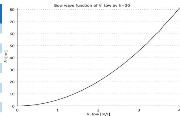
Figure 79 Bow wave as a function of towing velocity
