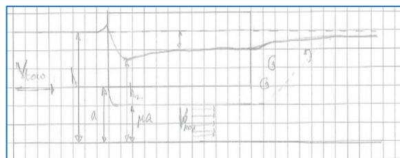
Figure 80 pressure drop under the tunnel element during the transport (B.P. Rigter, April 1989)
