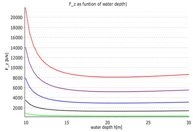
Figure 83 Vertical force as function of the water depth for five towing velocities (green = 0.5, black =1, blue=1.5, purple =2, red =2.5) in [m/s]
