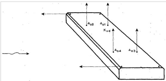
Figure 35 Vertical forces in the 4 suspension cables (W.D. Eysink, maart 1981)
