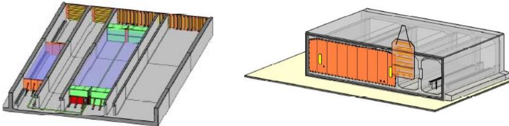
Figure 10 Principle of installing ballast tanks and bulkheads (FEHMARN BELT CONTRACTORS, 2013)
