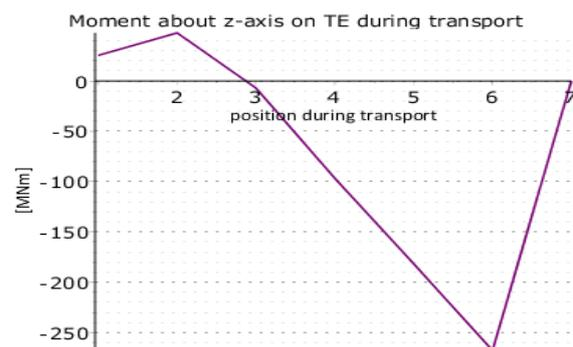
Figure 78 Moment on TE about the z-axis during different transport stages
