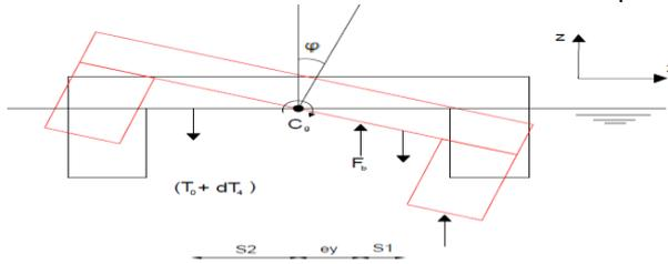
Figure 104 displacement in the roll degree of freedom
