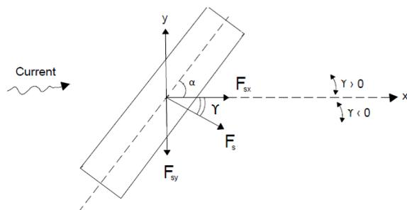
Figure 68 Transversal force in the y-direction
