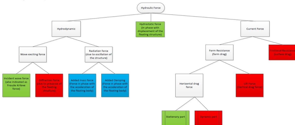
Figure 37 Overview of the Hydraulic forces during immersion
