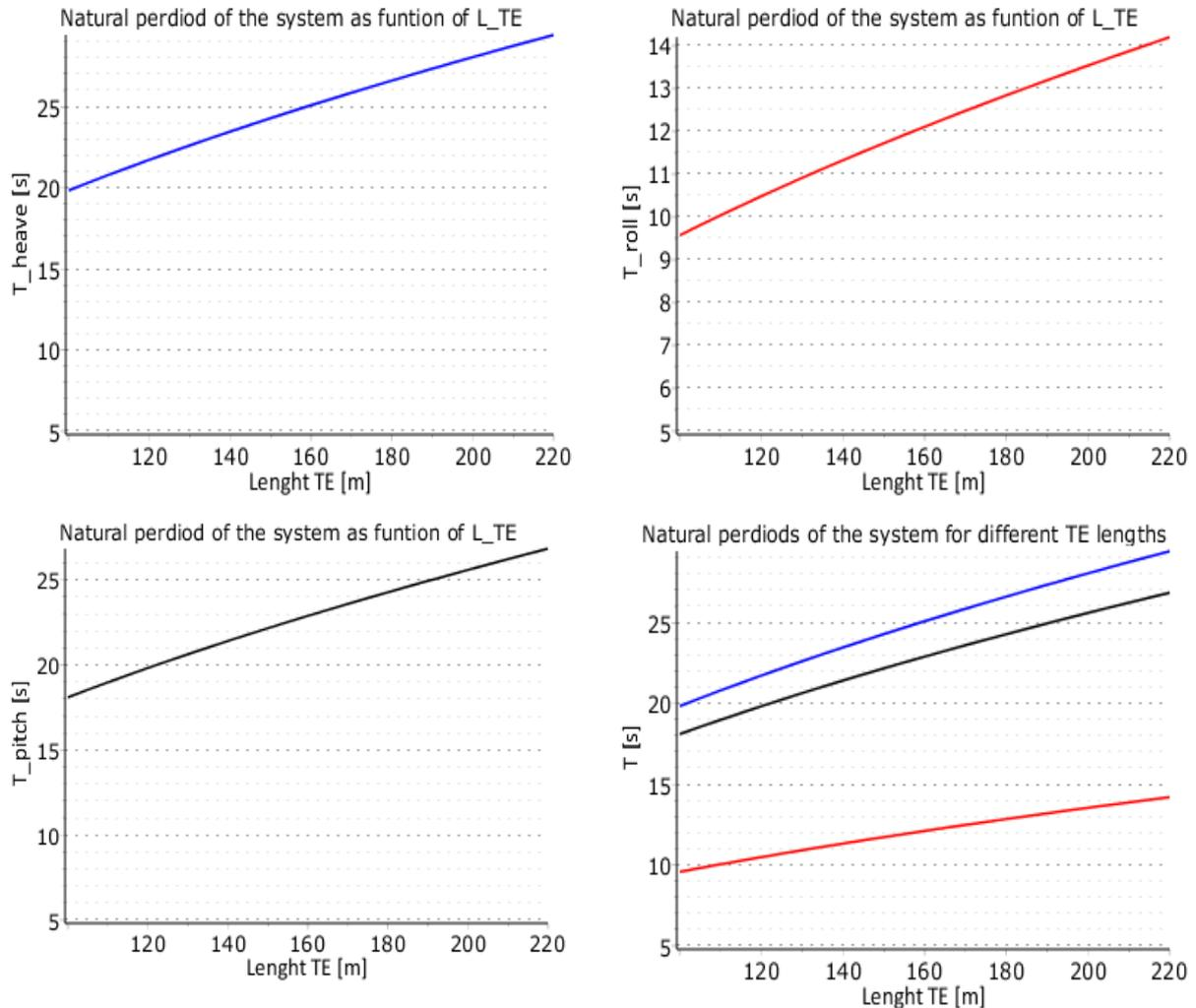
Figure 94 Natural periods of the system for the Catamaran pontoon for different lengths of TE (blue= heave; red=roll; black=pitch)
