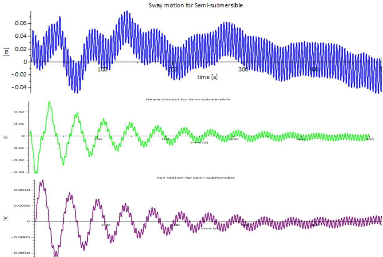
Figure 111 Motions of Semi-submersible in sway, heave and roll degrees of freedom for  $T_p=3.82$  [s] and  $H=2$  m
