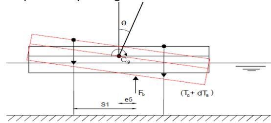
Figure 105 displacement in the pitch degree of freedom
