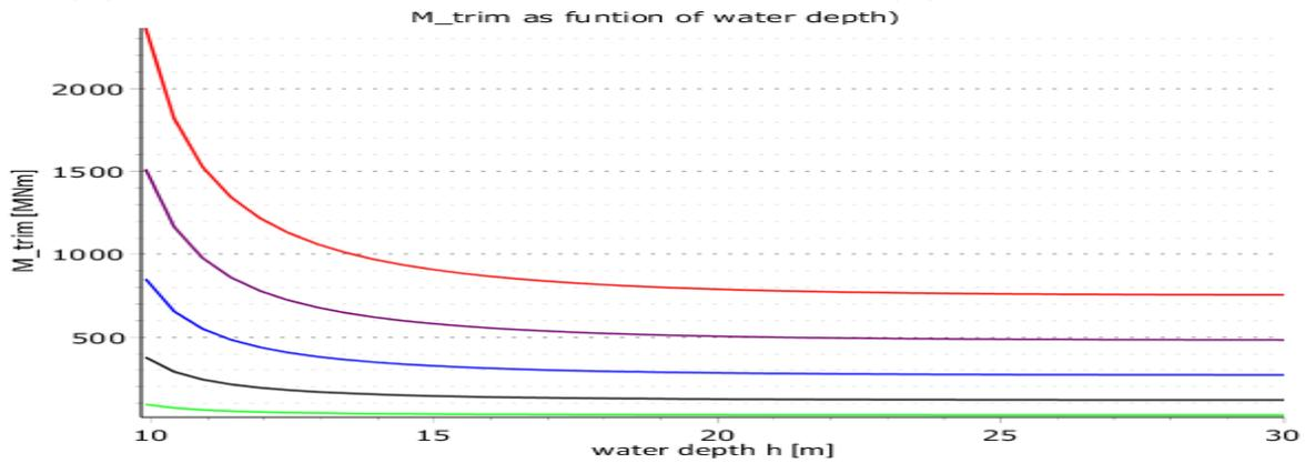
Figure 84 Trim moment as function of the water depth for five towing velocities (green = 0.5, black =1, blue=1.5, purple =2, red =2.5) in [m/s]
