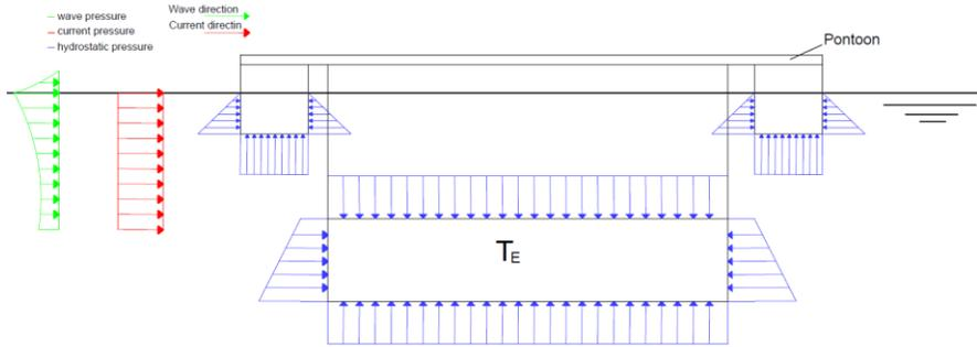
Figure 19 Main hydraulic forces working on the system
