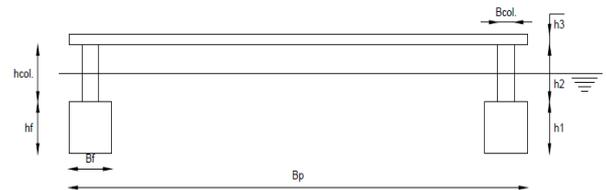
Figure 122 Semi-Submersible pontoon
