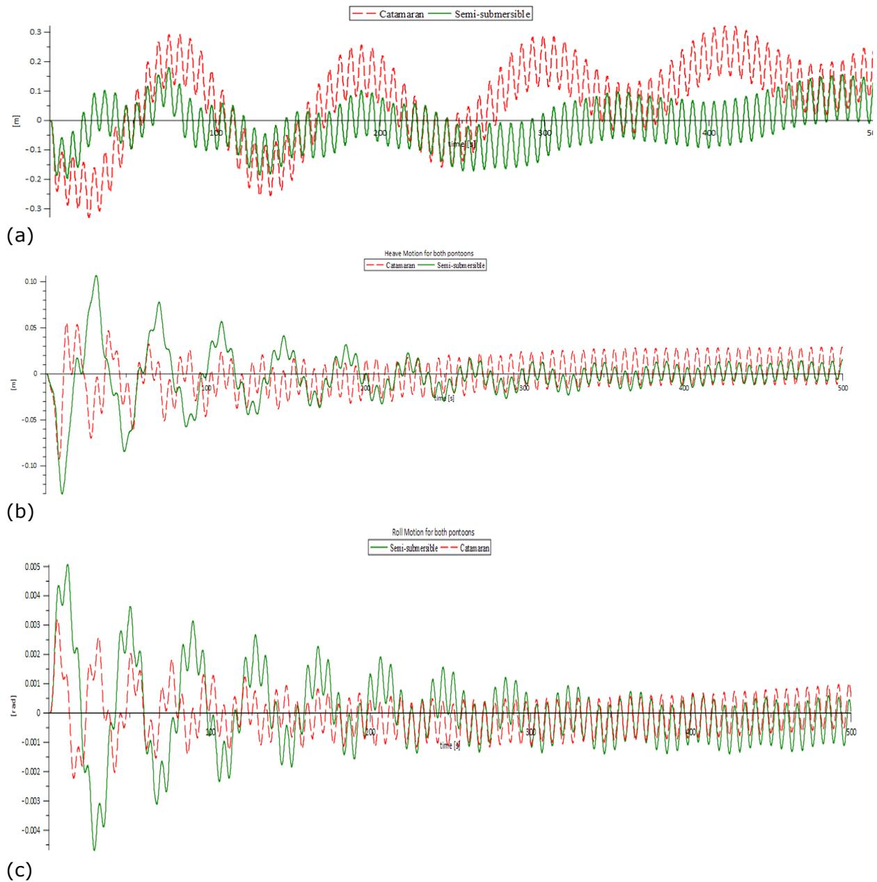
Figure 118 Motions of Catamaran and Semi-submersible pontoons in sway, heave and roll for  $T_p=6.5$  [s] and  $H_d=1.2$ m (4 suspension cables)
