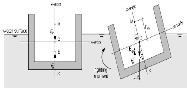
Figure 45 Static stability of the TE during the transport (M.Z. Voorendt, W.F. Molenaar, K.G. Bezuyen, 2011)
