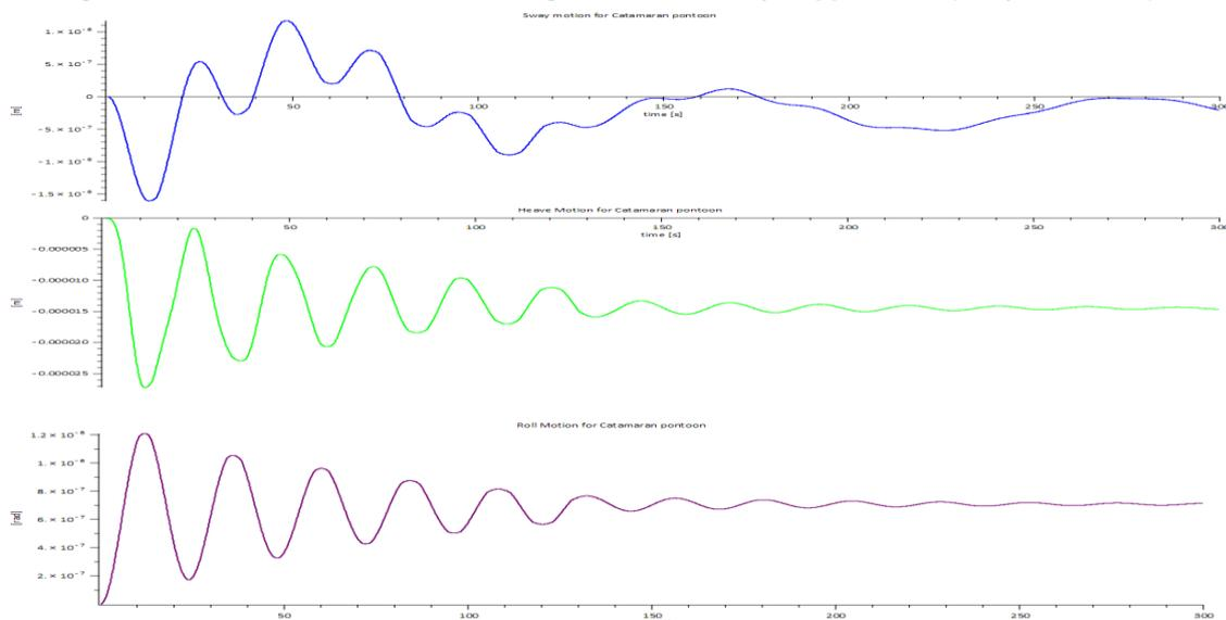
Figure 116 Motions of Catamaran Pontoon in 6 degrees of freedom for  $T_p=0.80$  [s] and  $H=1m$  (2 suspension cables)
