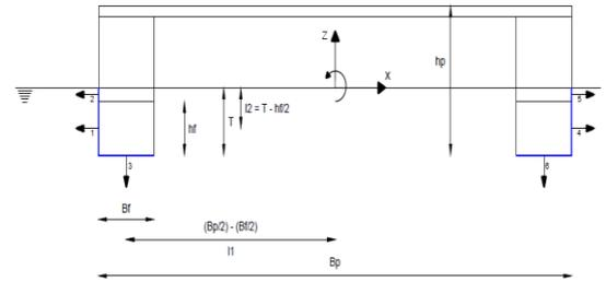
Figure 125 parts of the pressure integration for the wave force calculations
