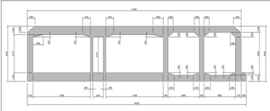
Figure 39 Actual cross-section tunnel element (Femern A/S, 2013)
