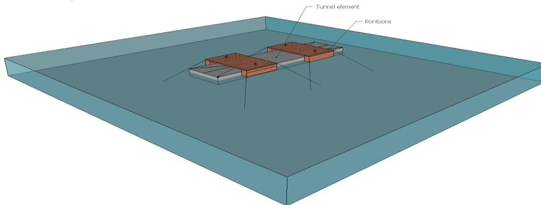
Figure 4 Tunnel element and two pontoons (also indicated as system)
