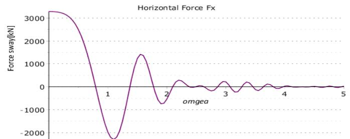
Figure 128 Sway force on the Semi- submersible
