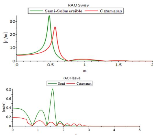
Figure 138 RAO's for Semi-submersible and Catamaran pontoon
