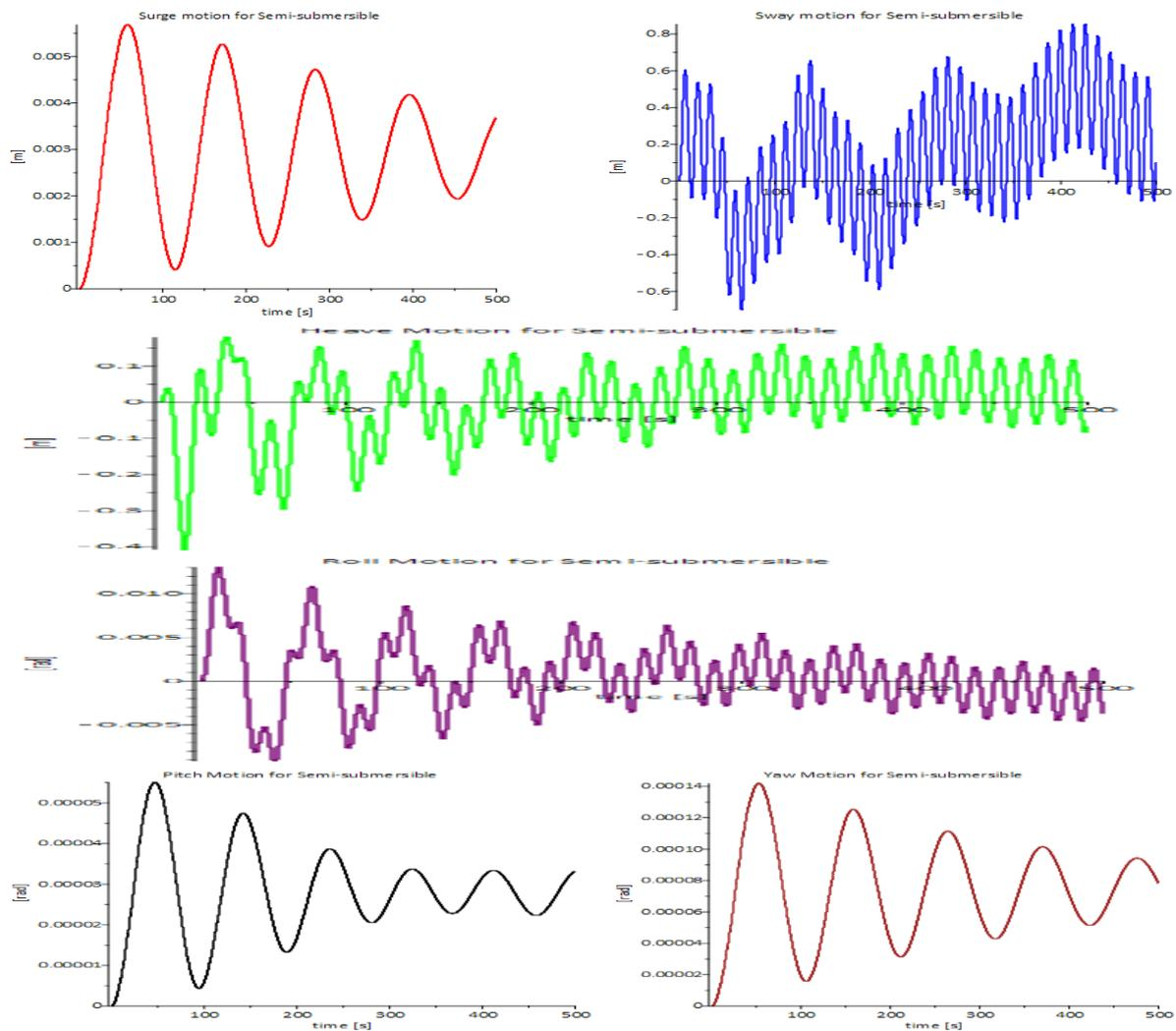
Figure 113 Motions of Semi-submersible in 6 degrees of freedom for  $T=13$  [s] and  $H=1\text{m}$  (2 suspension cables applied)
