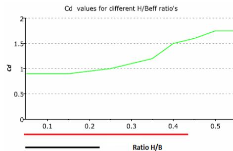
Figure 64 Drag Coefficient as function of  $H/B$
