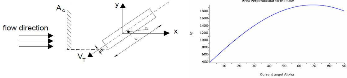
Figure 60 Area perpendicular to the current direction
