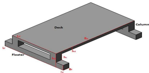
Figure 44 Semi-submersible pontoon
