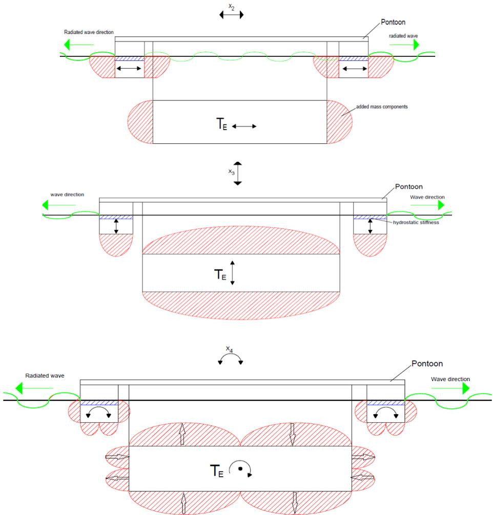
Figure 20 Extra forces on the system due to dynamic movements of the surrounding water
