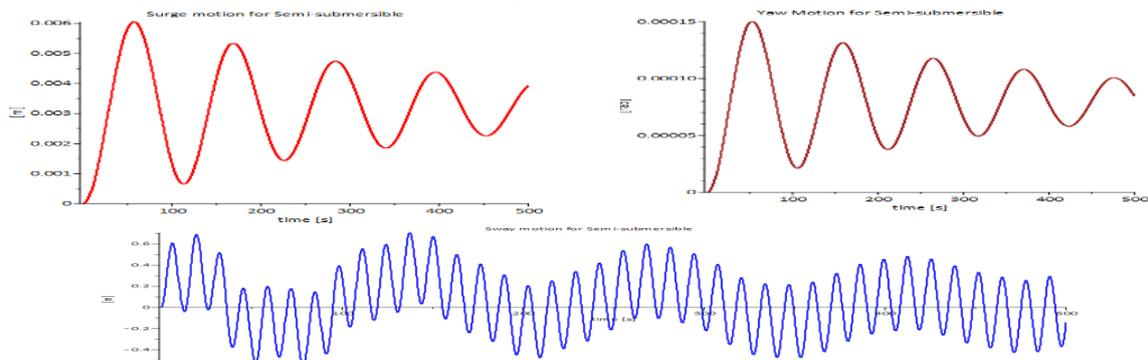
Figure 108 Motions of Semi-submersible in 'soft' degrees of freedom for  $T_p=13$  [s] and  $H=1m$
