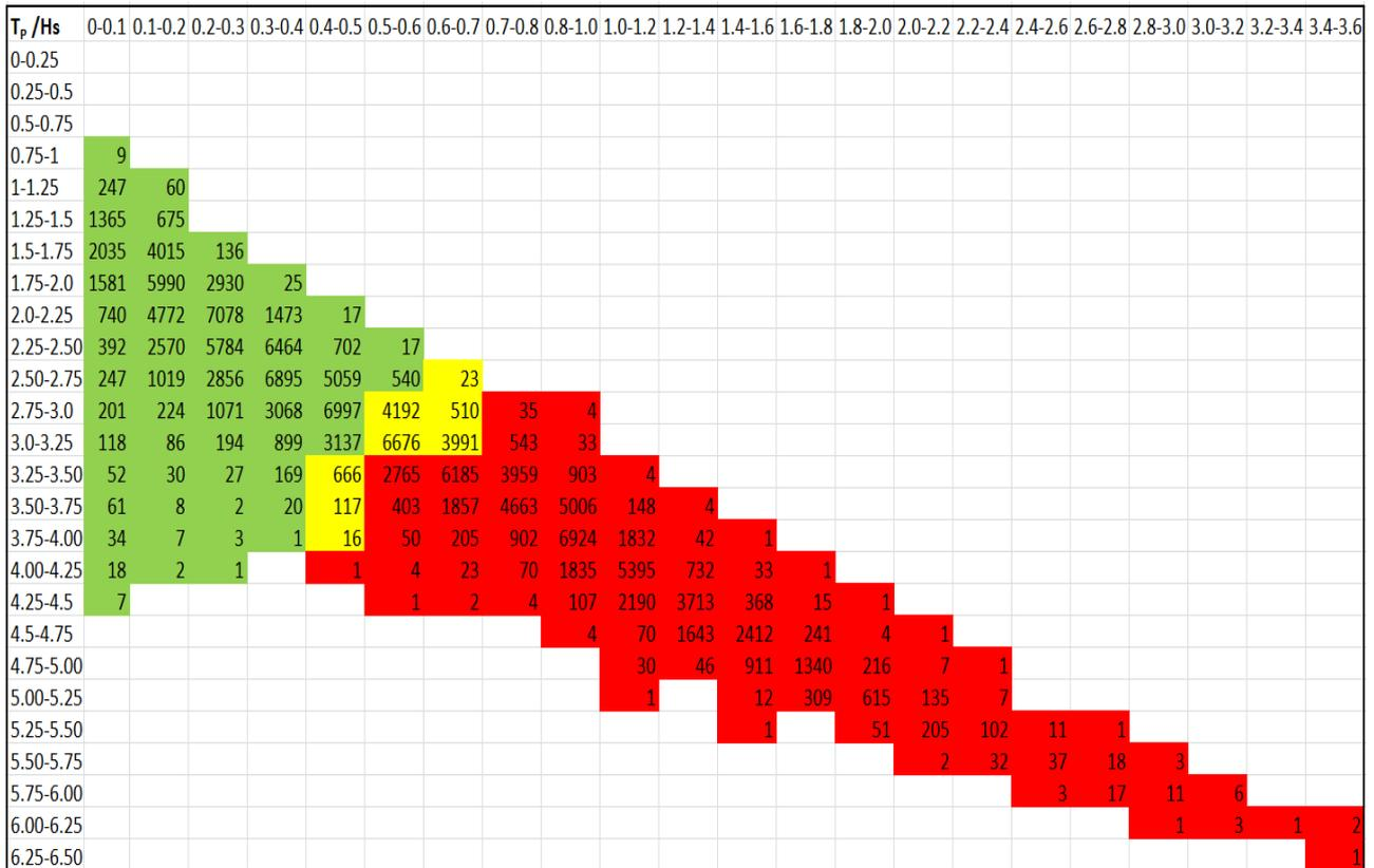
Figure 132 Workable conditions Semi-submersible pontoon (4 suspension cables applied)
