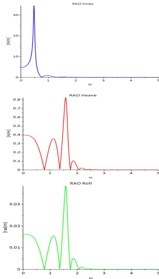
Figure 130 RAO's Semi-submersible pontoon in sway, heave and roll
