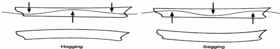
Figure 24 Principle of sagging and hogging conditions.<sup>1</sup>
