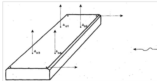
Figure 36 Vertical forces in the 4 suspension cables (W.D. Eysink, maart 1981)
