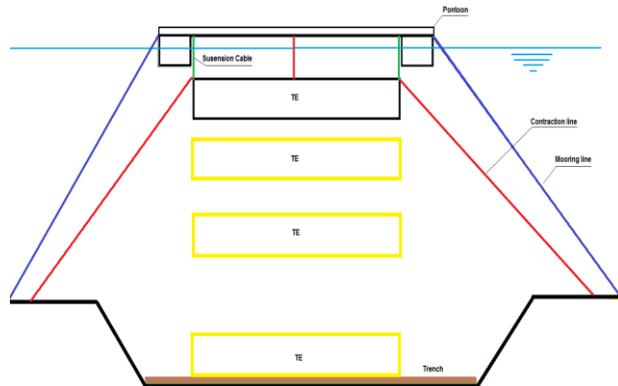
Figure 28 TE during immersion
