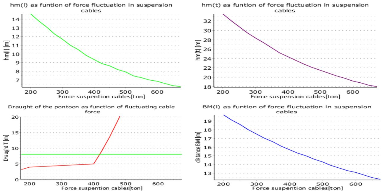
Figure 50 Static stability Semisubmersible pontoon
