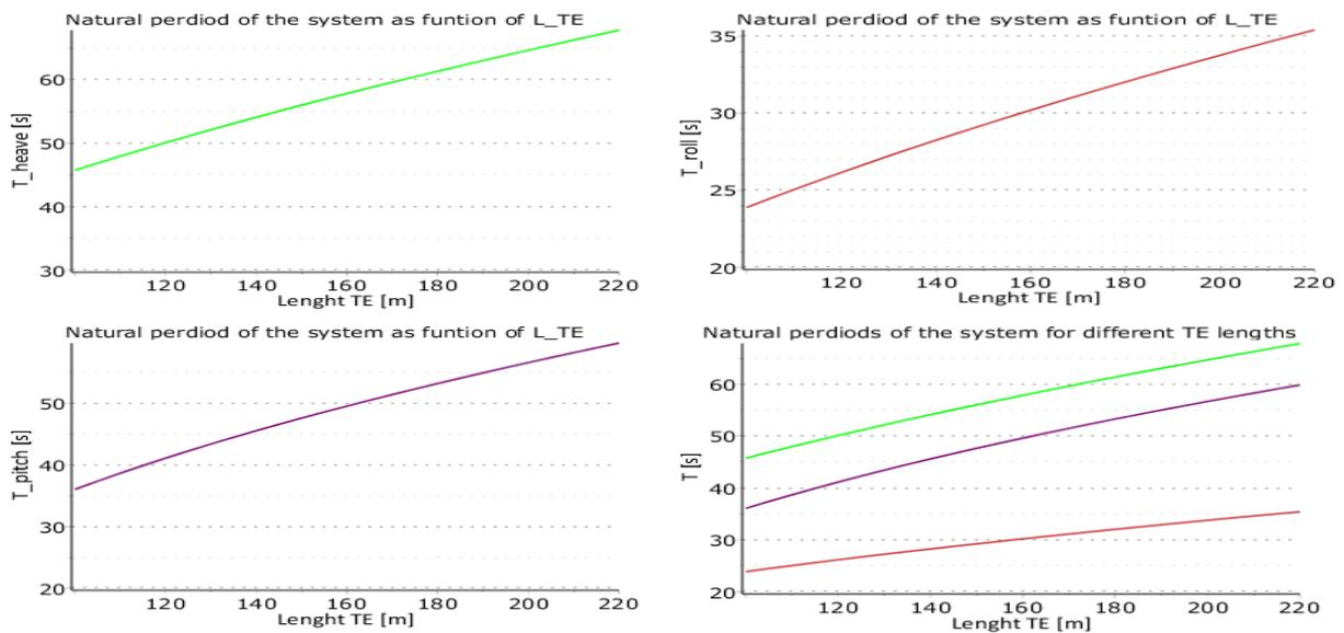
Figure 95 Natural periods of the system for the Semi-submersible type pontoon for different lengths of TE (green= heave; orange=roll; dark purple=pitch)
