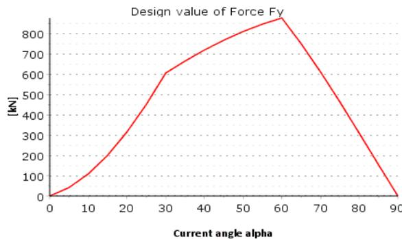
Figure 71 Design values of Force  $F_y$  as a function of the current angle  $\alpha$
