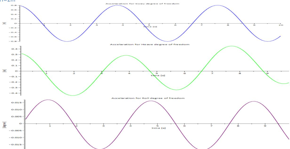
Figure 112 Accelerations of Semi-submersible in sway, heave and roll degrees of freedom for  $T_p=1.4$  [s] and  $H=2$  m
