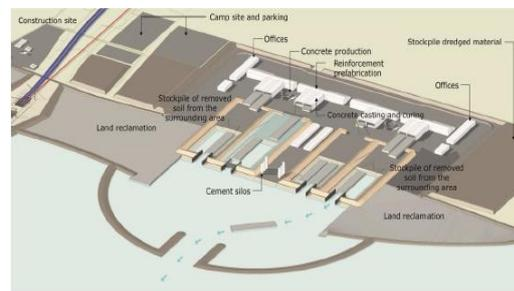
Figure 52 Schematic of tunnel production factory (Femern A/S, 2013)
