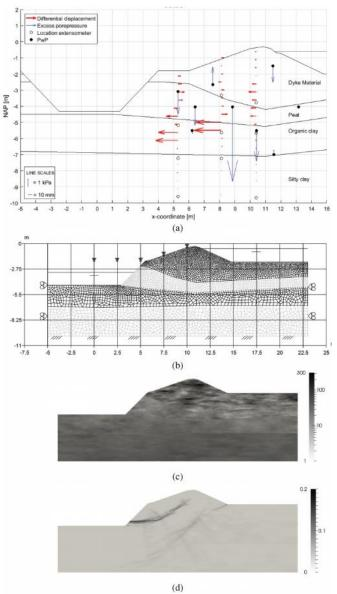
Figure 1. Analysis of the embankment: (a) measured differential displacements and excess pore pressures at the moment of failure; (b) finite element mesh used for analysis, with triangles indicating CPT locations, water level in ditch at NAP –3.15 m and waterlevel upstream at NAP –0.6 m; (c) example of an RFEM analysis, with shear strength illustrated on a logarimic scale in kPa (d) the calculated shearbands as contours of deviatoric strain.
