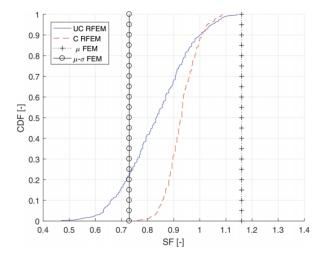
Figure 2. Analyses results for safety factor (SF).
