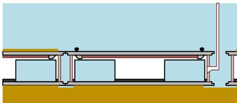
C.7 Float catamaran pontoons above the tunnel element and connect lifting lines.
