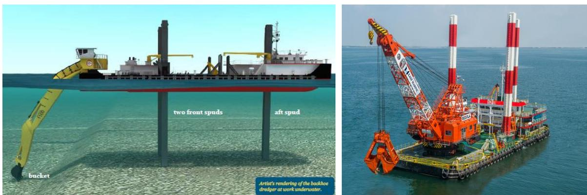
FIGURE 23, DREDGING EQUIPMENT (TEC, 2017)
