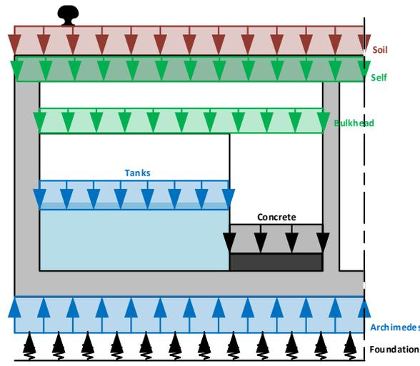
FIGURE 109, VERTICAL BALANCE CALCULATION; SITUATION SKETCH LOAD CASE V-III
