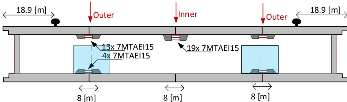
FIGURE 133, POST-TENSIONED PRESTRESSING LAY-OUT; LONGITUDINAL VIEW
