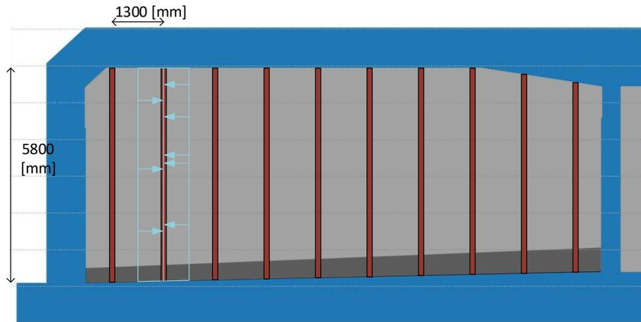
FIGURE 55, LOAD DISTRIBUTION ON BULKHEADS, CROSS-SECTION VIEW
