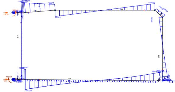
FIGURE 84, SHEAR LOAD COMB. A
