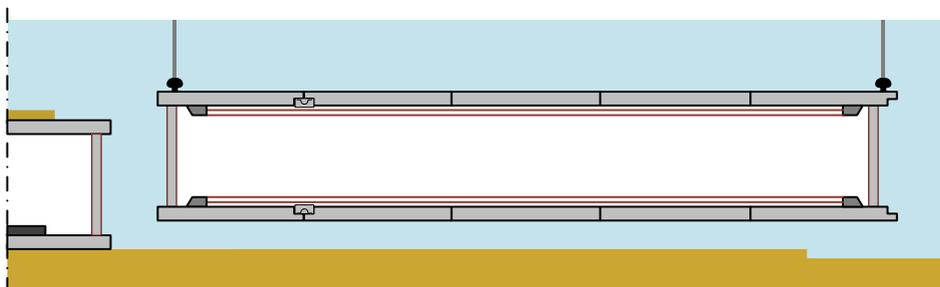
FIGURE 19, LIFTING MULTIPLE ELEMENTS, INCLUDING PRESTRESSING; LONGITUDINAL VIEW
