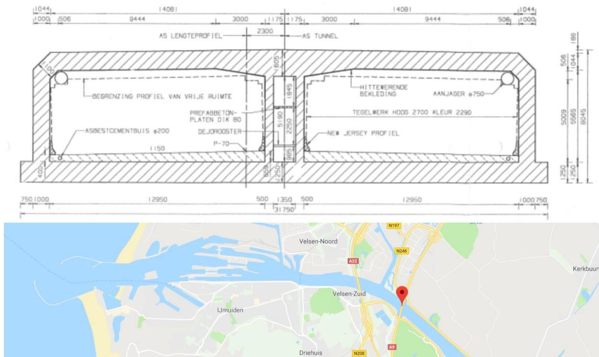
FIGURE 106, WIJERTUNNEL CROSS SECTION AND LOCATION
