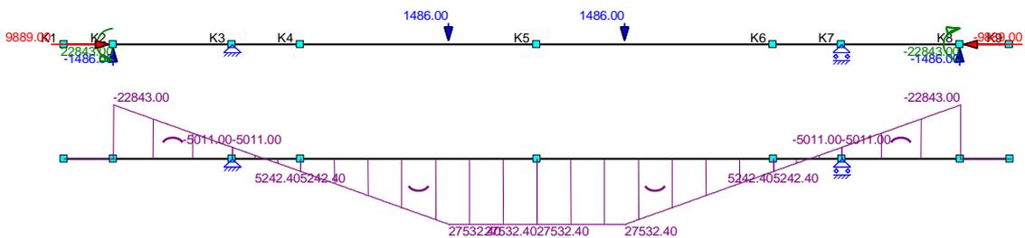
FIGURE 132, PRESTRESSING MODEL VARIANT 3 INPUT
