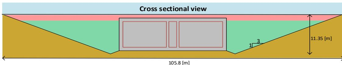
FIGURE 71 CROSS-SECTIONAL DREDGING SCHEME; CROSS-SECTION VIEW
