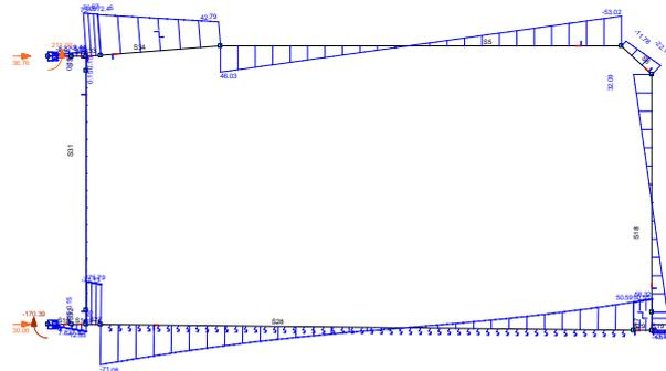
**FIGURE 118, SHEAR CHANGE; WATER INCREASE (PER METER)**
