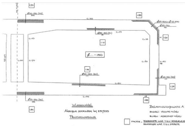
**FIGURE 51, TUNNEL CROSS-SECTIONAL REINFORCEMENT (PRELIMINARY)**
