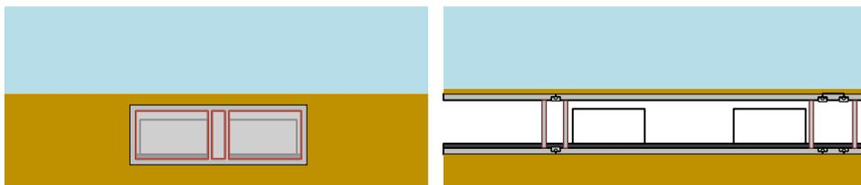
A.6 Pump in ballast water to a base level resulting from the buoyancy calculations. The ballast system must be controlled remotely by pneumatic or hydraulic valves.
