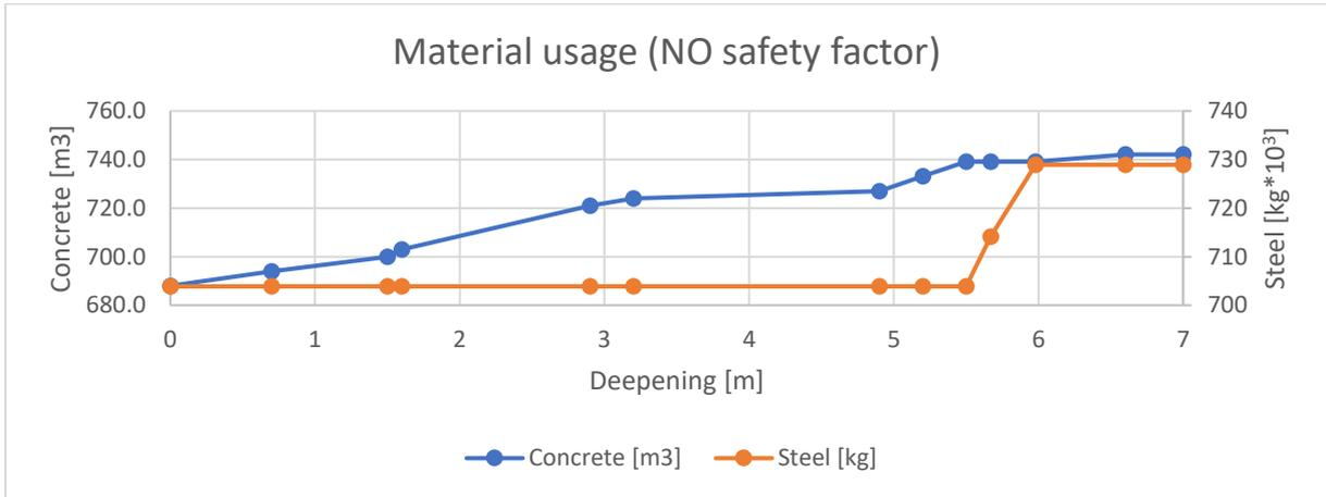
FIGURE 87, MATERIAL USAGE WITHOUT SAFETY FACTORS
