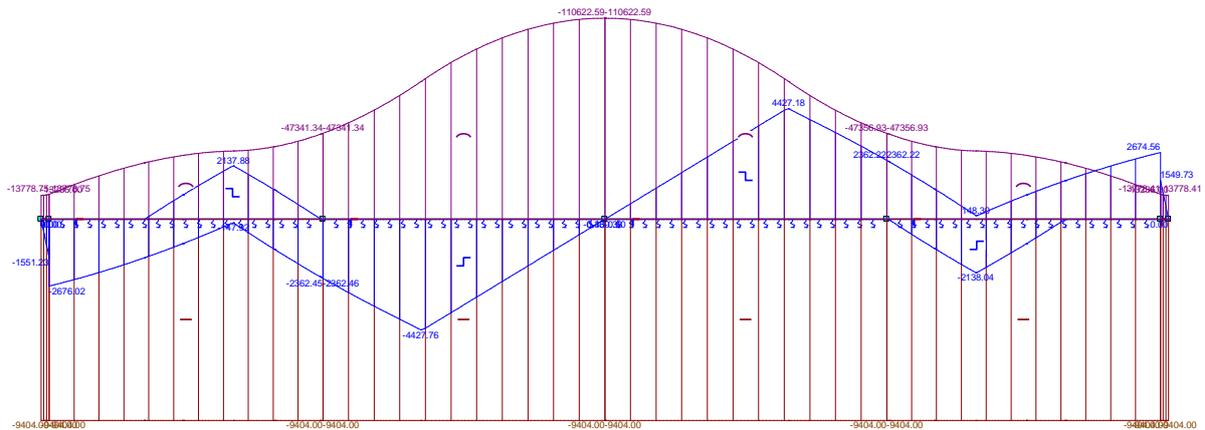
FIGURE 128, PRESTRESSING MODEL RESULTING ENVELOPE CASE D.1+E.1+F.1
