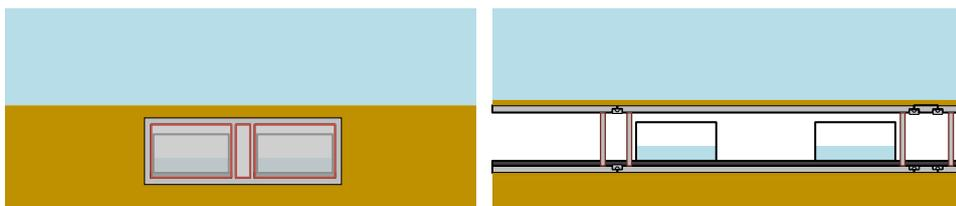
A.7 Remove ballast concrete; depending on the design step 6&7 are carried out in multiple phases.
