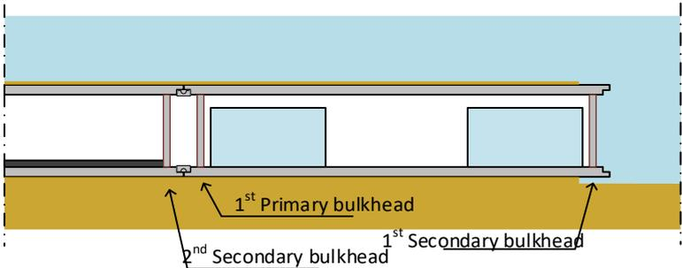
FIGURE 13, BULKHEAD FAILURE SAFETY, LONGITUDINAL VIEW
