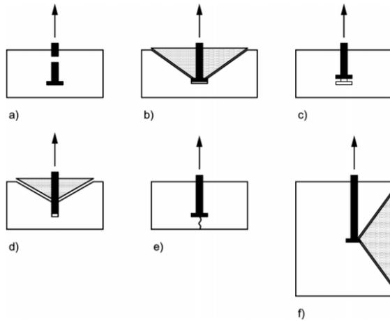
FIGURE 111, TENSION FAILURE MODES
