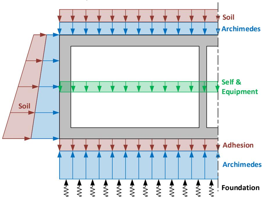
FIGURE 45, CROSS-SECTION VIEW INCLUDING LOADS
