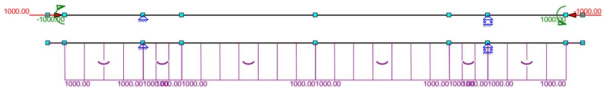
FIGURE 130, PRESTRESSING MODEL VARIANT 1 INPUT
