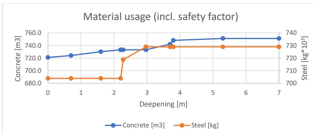
FIGURE 56, MATERIAL USAGE BULKHEADS
