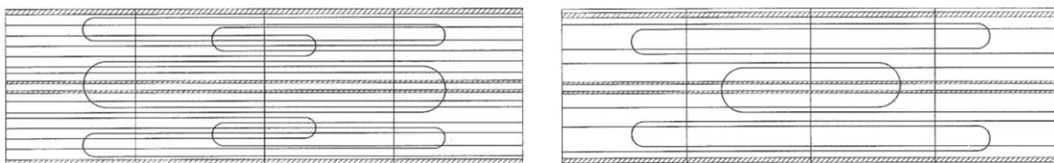
**FIGURE 21, PRESTRESSING DIAGRAM IN THE WIJKER TUNNEL (LEFT IS THE ROOF, RIGHT IS THE DECK)**
