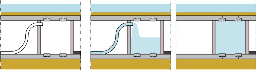
FIGURE 12, BULKHEAD WATERTIGHT TESTING PHASING; LONGITUDINAL VIEW
