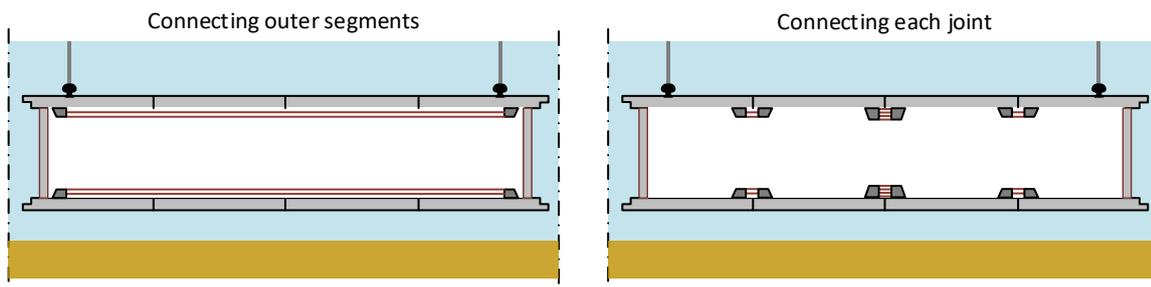
**FIGURE 20, PRESTRESSING DESIGN VARIANT (1/2) ; LONGITUDINAL VIEW**
