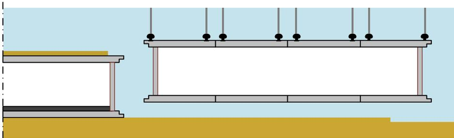
FIGURE 17, LIFTING MULTIPLE SEGMENTS TOGETHER; LONGITUDINAL VIEW
