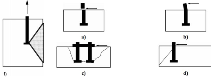
FIGURE 112, SHEAR FAILURE MODES
