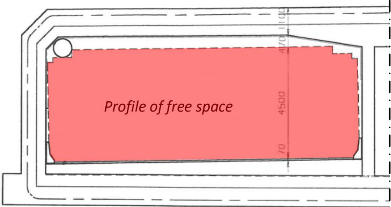
FIGURE 85, WIJKERTUNNEL PROFILE OF FREE SPACE; CROSS-SECTION VIEW
