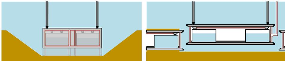
C.12 When the element approaches the water level gradually the ballast water tanks are emptied.
