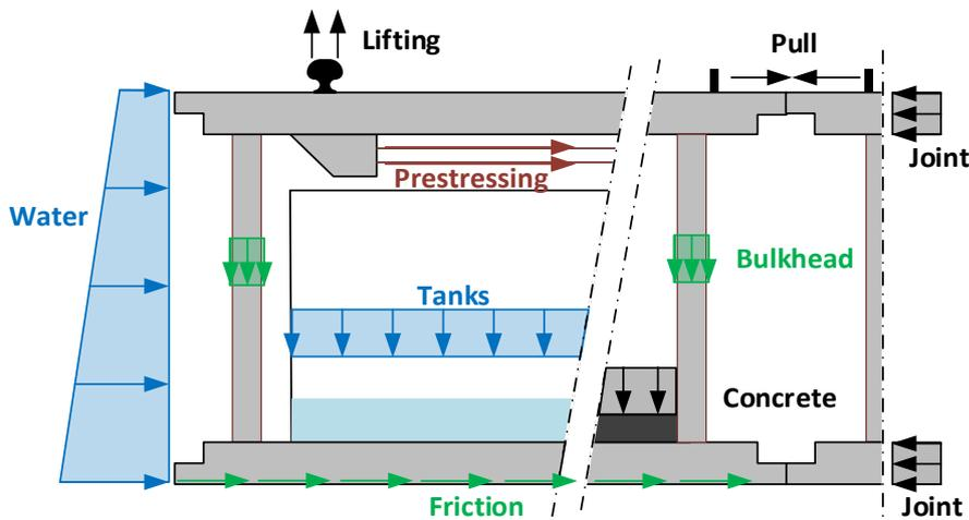
FIGURE 44, LONGITUDINAL VIEW INCLUDING FORCES
