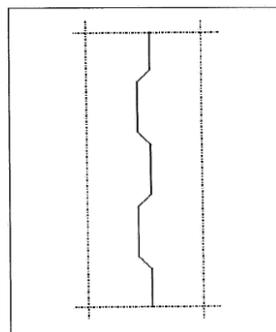
FIGURE 60, WIJKER TUNNEL SHEAR KEYS (CAMERIK & LEEUW, CEMENT, 1994)
