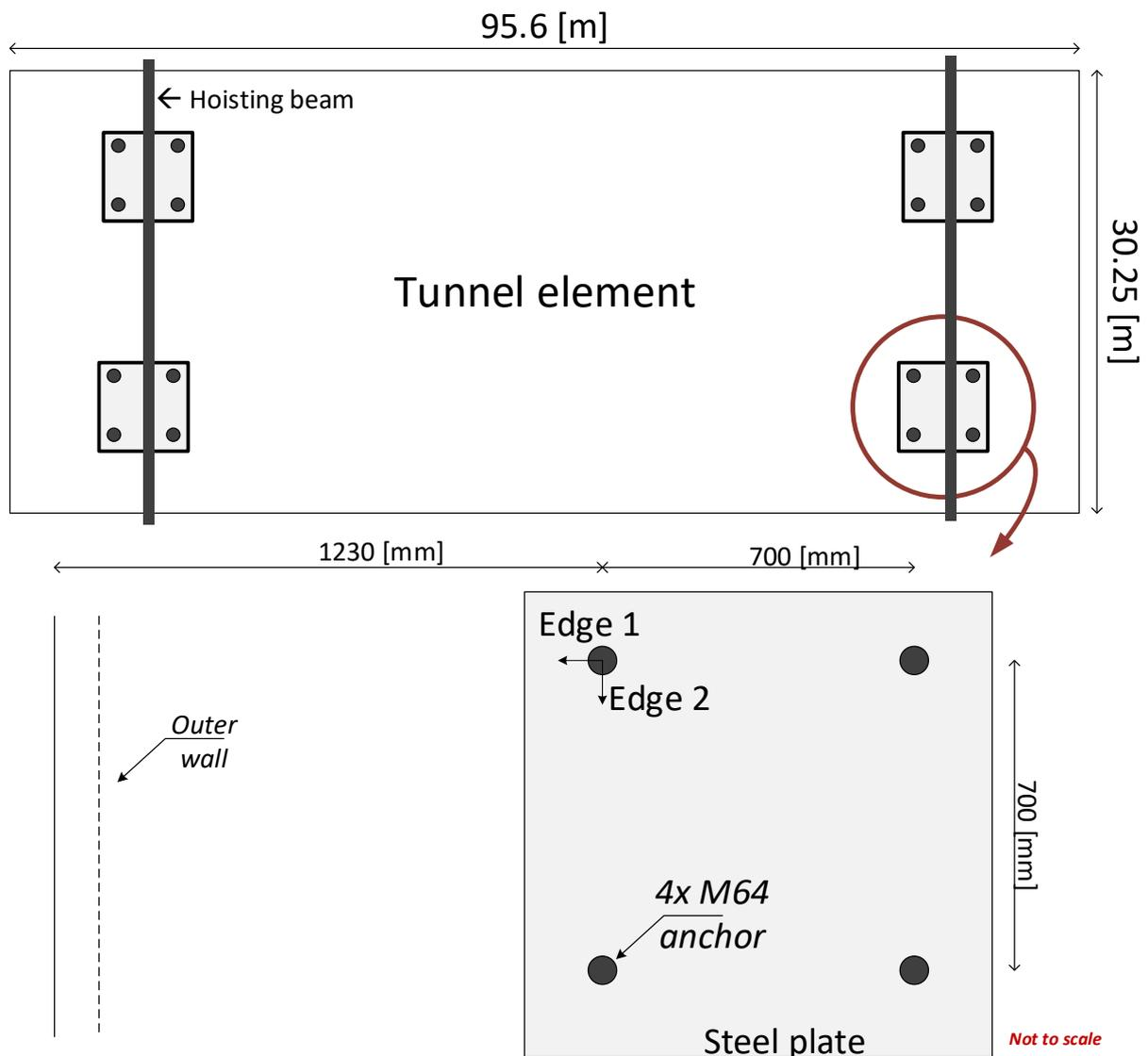
FIGURE 57, ANCHOR LAYOUT TUNNEL ROOF; TOP VIEW
