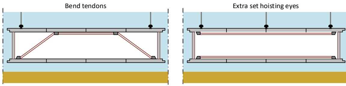
**FIGURE 22, PRESTRESSING DESIGN VARIANTS (2/2) ; LONGITUDINAL VIEW**
