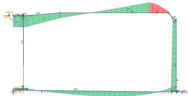
FIGURE 59, HOISTING MOMENTS IN CROSS-SECTION
