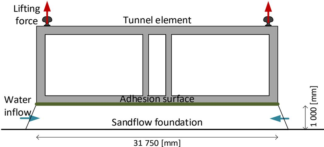
FIGURE 27, SOIL ADHESION SITUATION SKETCH
