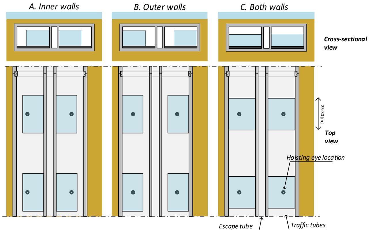
FIGURE 10, BALLAST TANK DESIGN LAY-OUTS
