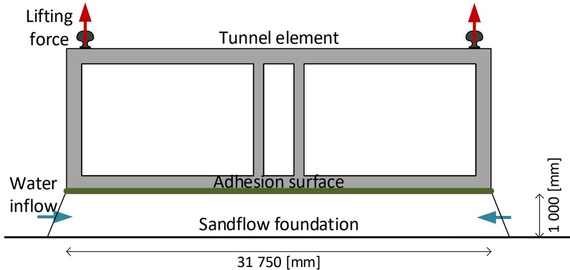
FIGURE 113, SOIL ADHESION SITUATION SKETCH; CROSS SECTIONAL VIEW
