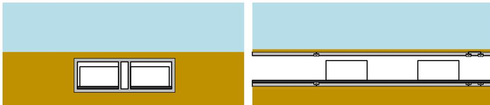
A.5 Install bulkheads; on one end the bulkhead may be accommodated with a docking station to connect an access shaft (after cutting)
