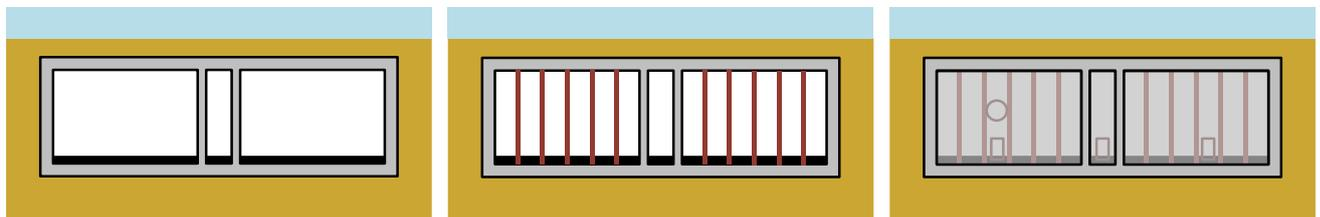
FIGURE 11, BULKHEAD CONSTRUCTION PHASING; CROSS-SECTIONAL VIEW
