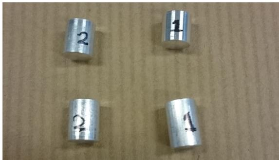
(a) Samples used to estimate the thickness of the glue
