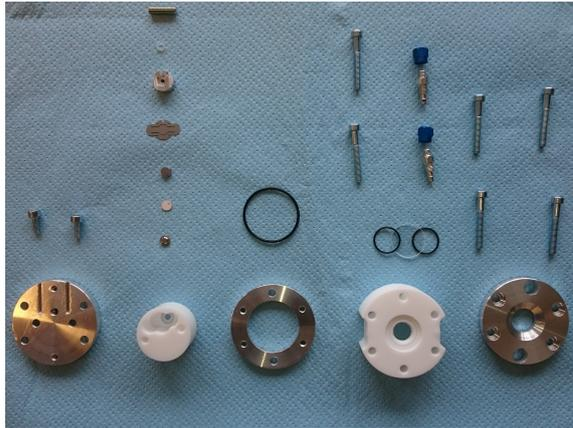
(a) Fabricated components and vendor parts, displayed from left to right the components from the bottom to the top
