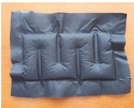
Figure 94: High frequency sealed pad
