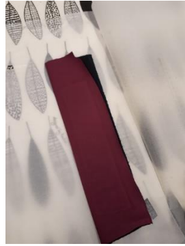
Figure 54: Bonding fabrics together with PU hotmelt tape
