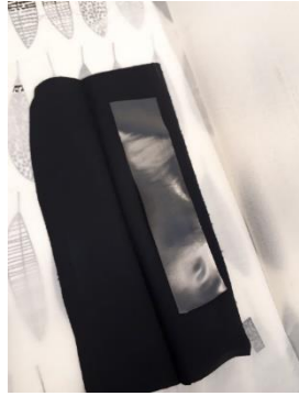
Figure 54: Bonding fabrics together with PU hotmelt tape
