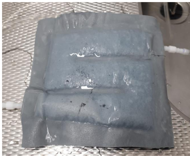
Figure 103: Pad with evaporation fabric
