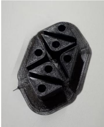
Figure 81: TPU printed connector
