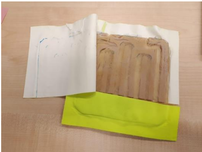
Figure 5: Opened delaminated pad
