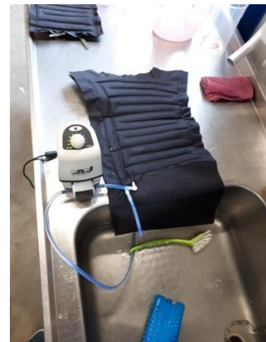
Figure 135: Testing for leaks
