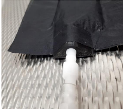
Figure 82: TPU connector melted in pad
