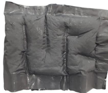
Figure 96: Finished pad with sealed bulkheads
