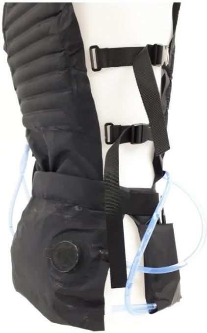
Figure 150: Detailed view of reservoir and tightening bands
