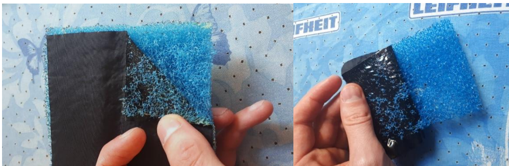
Figure 85: testing bond between fabric and foam
