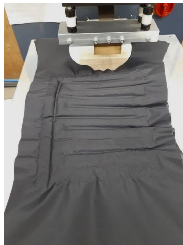
Figure 134: Sealing outer edge
