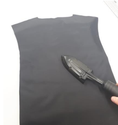
Figure 132: Melting fabric to foam
