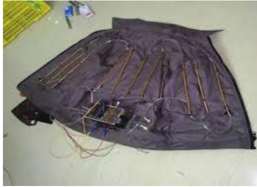
Figure 37 : Thermoelectric liquid circulation vest (Lavanya, 2016)
