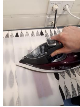
Figure 54: Bonding fabrics together with PU hotmelt tape
