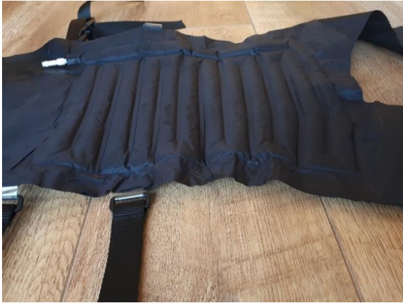
Figure 155: Shrinking and warping due to sealing lines
