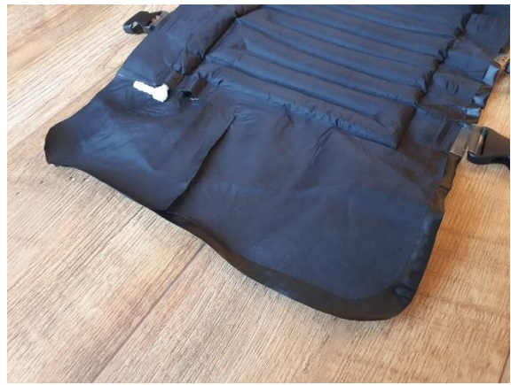
Figure 158: Misaligned fabric pieces
