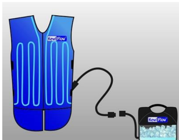
Figure 36: Active PCM cooling schematic (Triathlonaccessoires.nl, N.D.)
