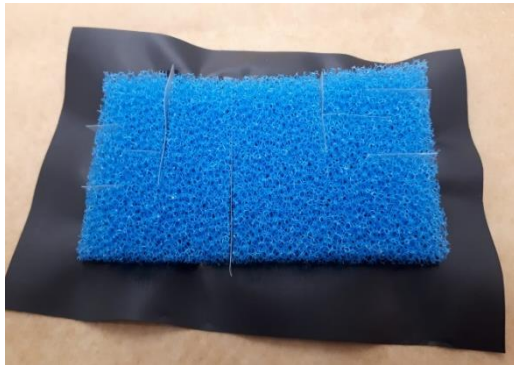
Figure 92: PU tape inserted in slits
