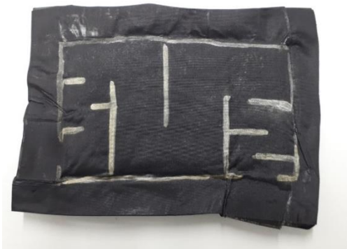
Figure 93: Finished pad with PU tape bulkheads
