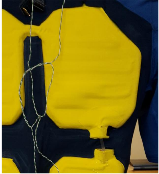
Figure 4: Delamination of the pad
