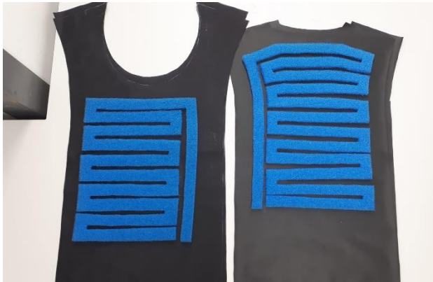
Figure 131: Panels with their foam pieces
