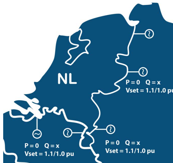
Figure 26: Border generator setup for forced border voltages.
