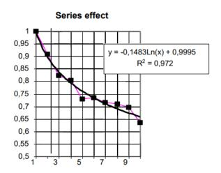
Figure A.2: Reduction of workload (series effect) from the first to the 10th ship
