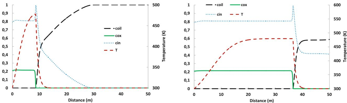
**Fig. 5** Simulation for HPAI into a porous media filled with oil of lower viscosity. Same variables are shown at the same times as in Fig. 2. Left y-axis shows the fraction
