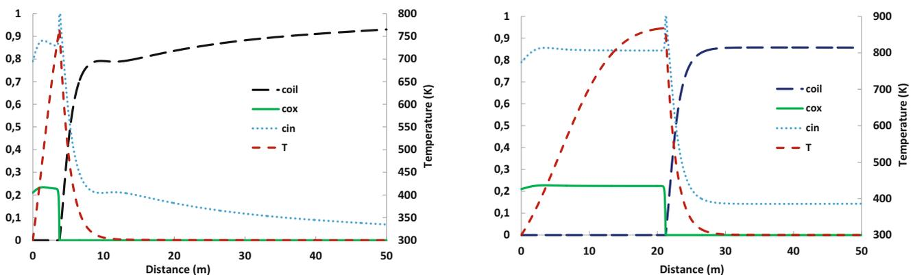
**Fig. 4** Simulation for HPAI into a porous media filled with oil of higher viscosity. Same variables are shown at the same times as in Fig. 2. Left y-axis shows the fraction
