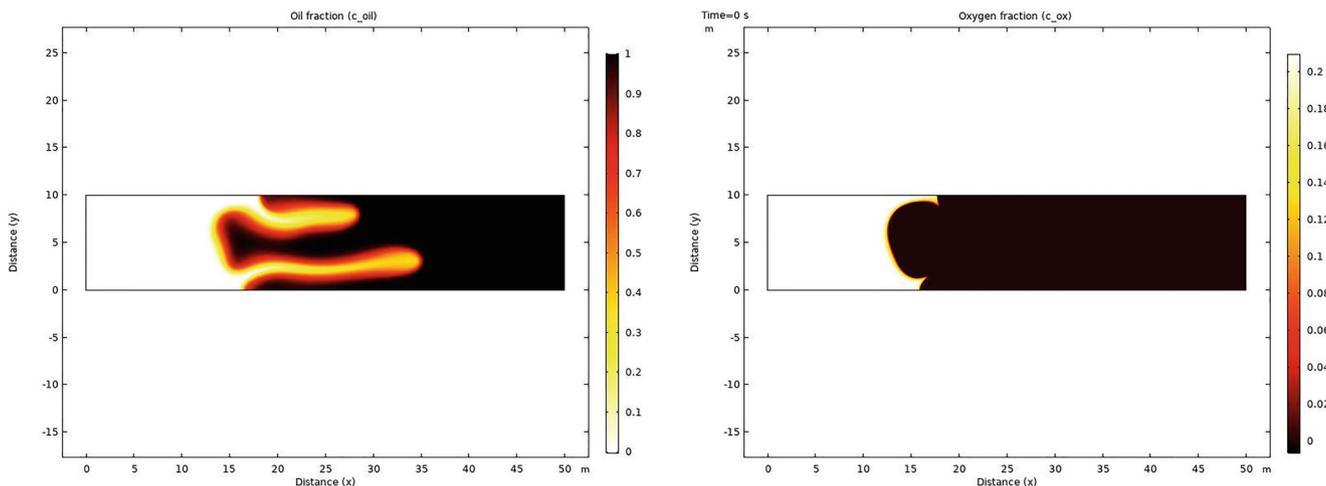
**Fig. 6** 2D simulation for HPAI into a porous media filled with oil. Indicated by color are the distribution of oil fraction  $c_{oil}$  (left) and oxygen fraction  $c_{ox}$  (right)
