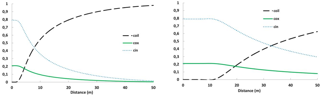
**Fig. 3** Simulation for HPAI into a porous media filled with oil when the reaction is not present. Same variables are shown at the same times as in Fig. 2. Left y-axis shows the fraction
