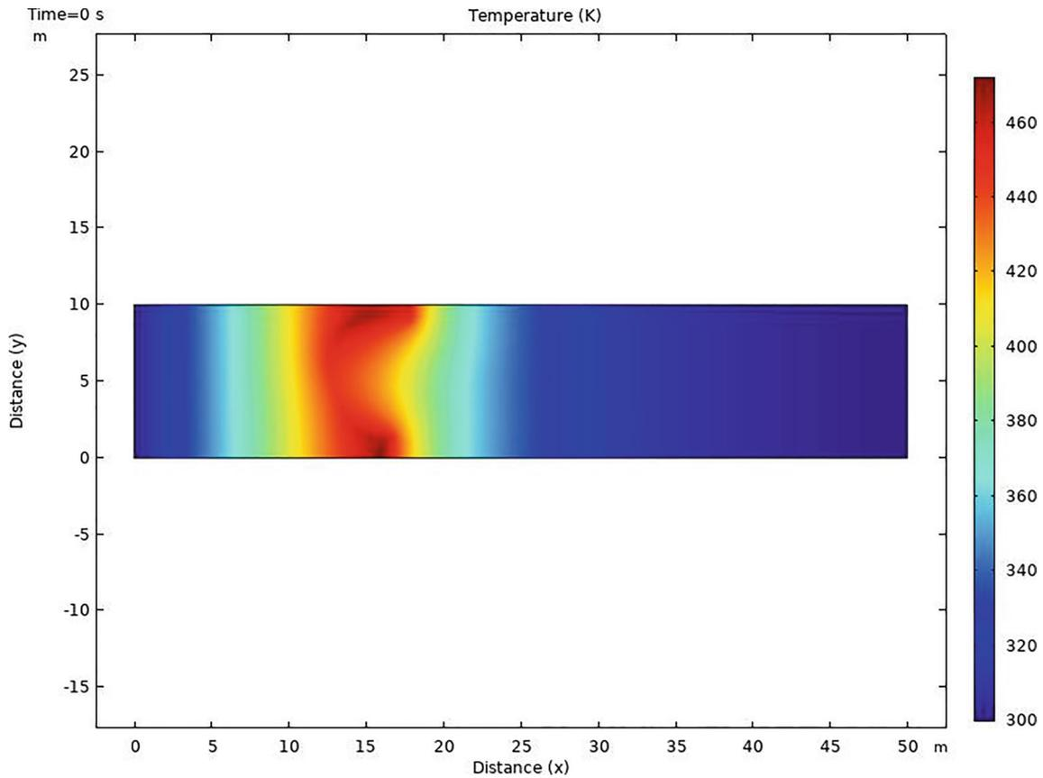
Fig. 7 2D simulation for HPAI into a porous media filled with oil. Indicated by color is the temperature  $T$
