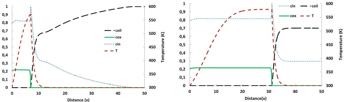
**Fig. 2** Simulation of HPAI into a porous media filled with oil. The left panel corresponds to the time  $t = 5 \times 10^6$  s, and the right panel to  $t = 2 \times 10^7$  s. Left y-axis shows the fraction. Indicated are the distributions of the temperature  $T$ , oil fraction  $c_{oil}$ , oxygen fraction  $c_{ox}$ , and
