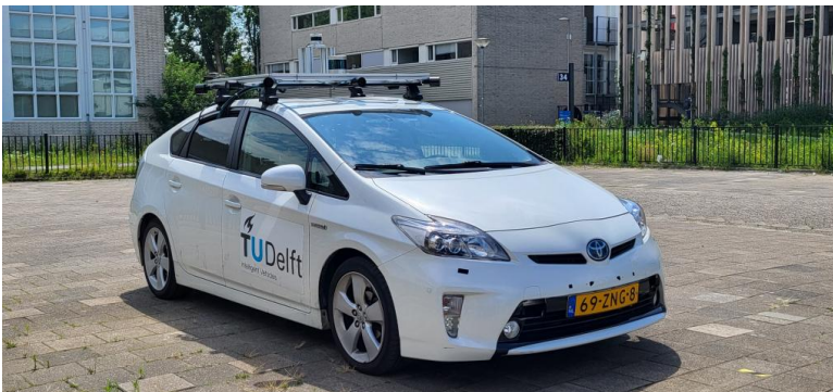
Figure 3.1: TU Delft experimental automated vehicle (third-generation Toyota Prius) used in the experimental validation.
