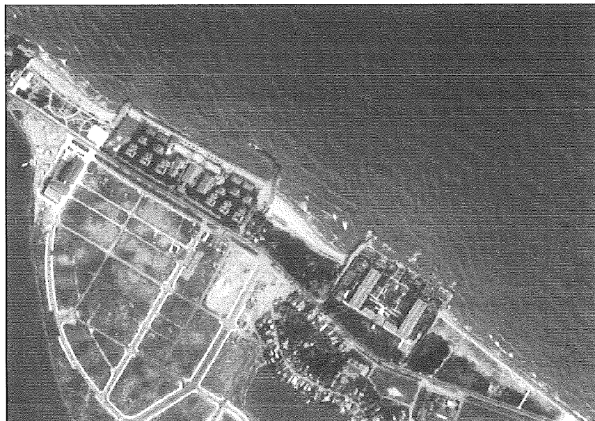
FIGURE 2.7: Severe beach erosion has occurred at the north side of the river mouth
