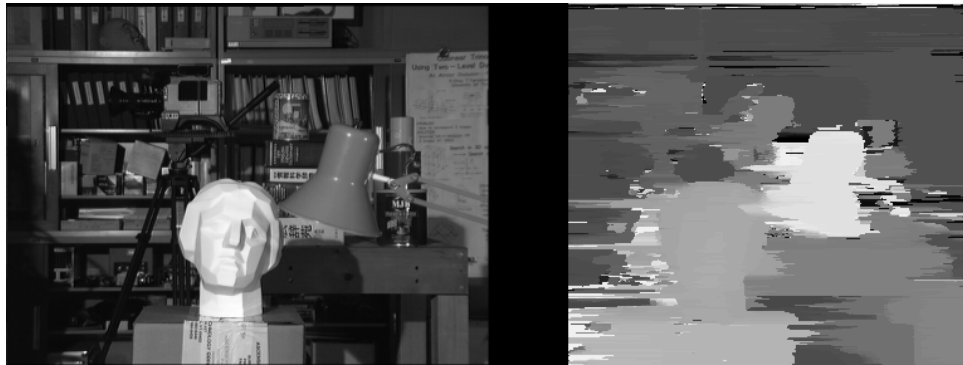
Figure 2. Tsukuba image from the Middlebury stereo benchmark and the resulting disparity map from our simplified implementation of [29].
