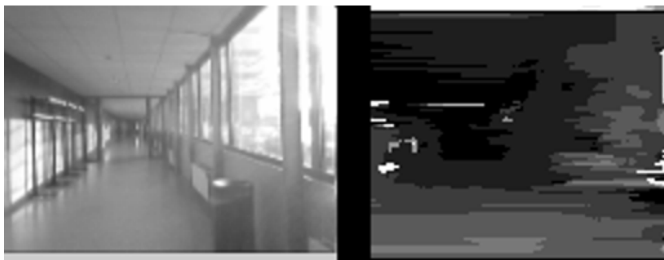
Figure 3. Result of the implemented stereo vision method (based on [29]) on images of a corridor, taken by the DelFly Explorer stereo vision camera.
