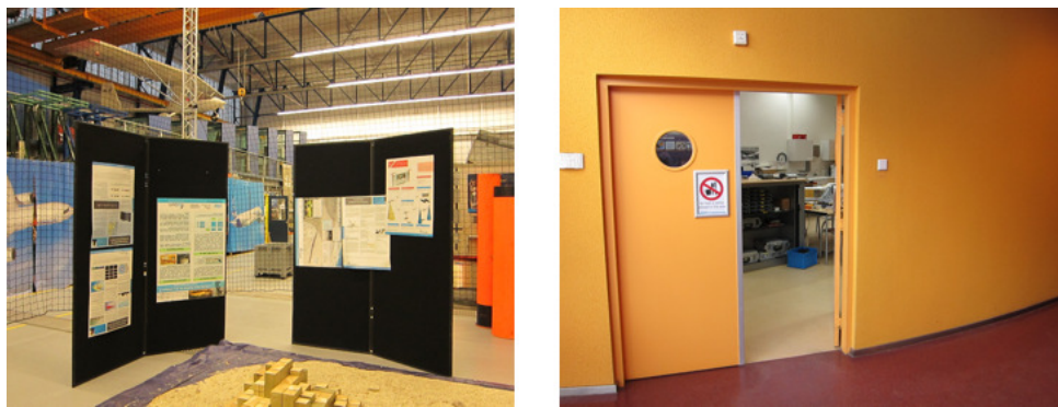
Figure 6. Experimental setup for flight tests with an opened door on the left. The gap between the black walls is 80 cm. The right image shows a real door used for testing.
