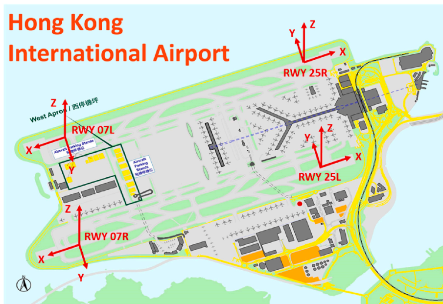
Fig. 11. Coordinate system transformation for HKIA.
