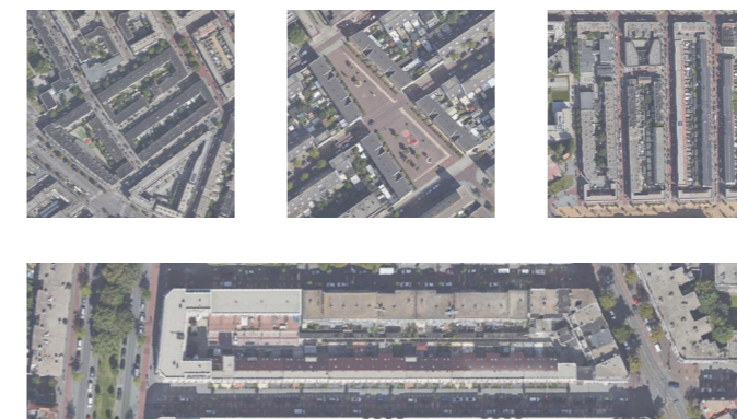
Figure 3.12. Satellite images that describe dark-colored roofs, impervious pavement, less vegetation and linear blocks (From left to right).
