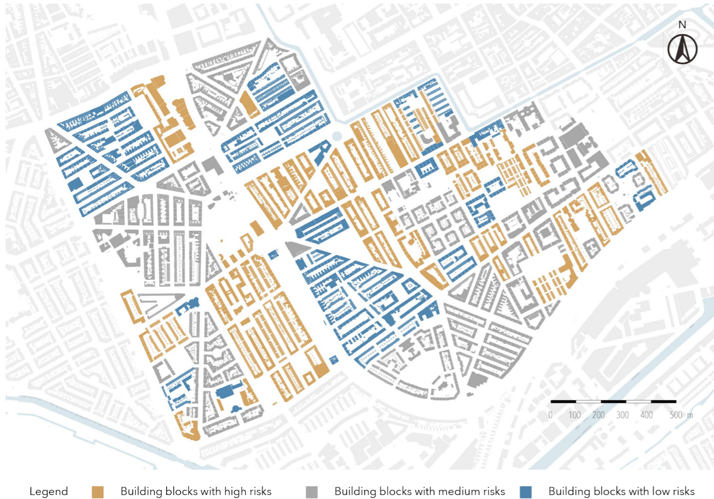
Figure 4.12. Risks map of building blocks from the perspectives of building configuration and microclimate.
