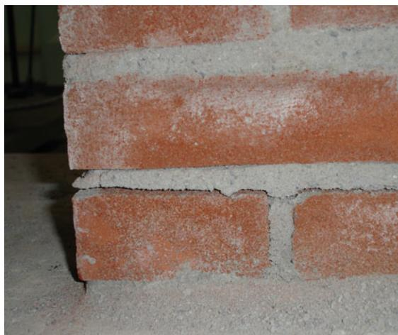
Figure 5.1: Tensile failure in masonry arch
