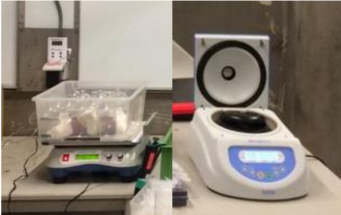
Figure 6: Set-up of batch experiment (left: shaker with sample bottles, right: centrifuge)
