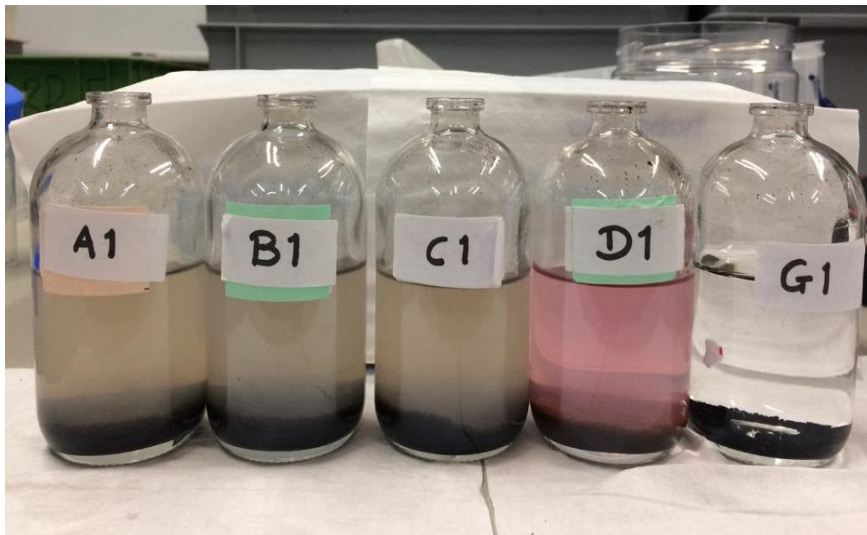
Figure 7: Sample bottles used for adsorption experiment (from left A1: Anaerobic aerated sludge with MPs 100 ug/l, B1: Anaerobic aerated sludge with MPs 200 ug/l, C1: Anaerobic aerated sludge with MPs 300 ug/l, D1: Anaerobic non-aerated sludge with MPs 100 ug/l, G1: GAC without sludge)
