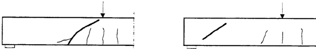
Figure 1.3, Flexural shear (left) and shear tension (right), (Walraven, 2002)
