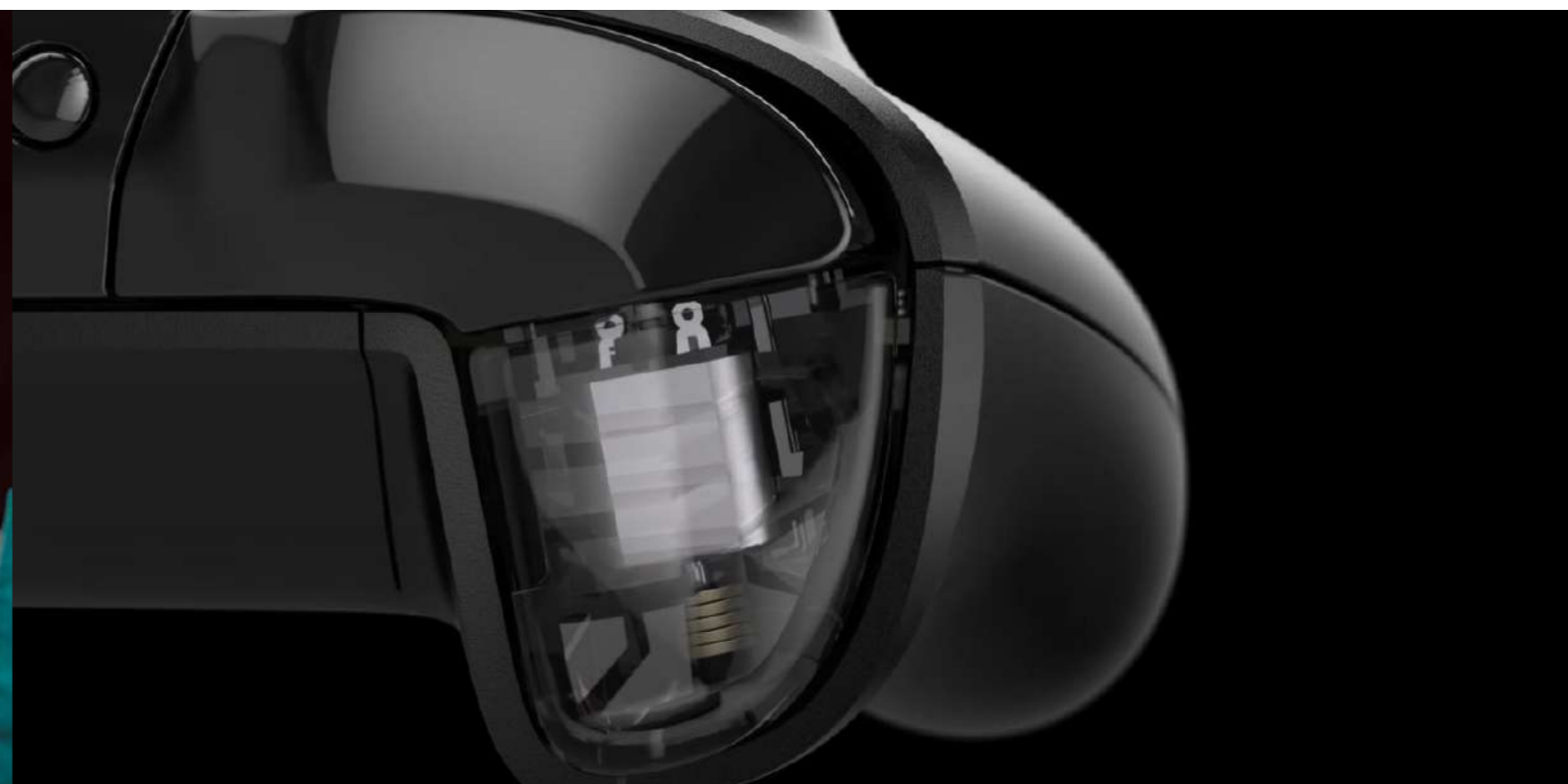
Figure 4 Haptic feedback in the trigger of gaming controllers (Xbox, 2013)
