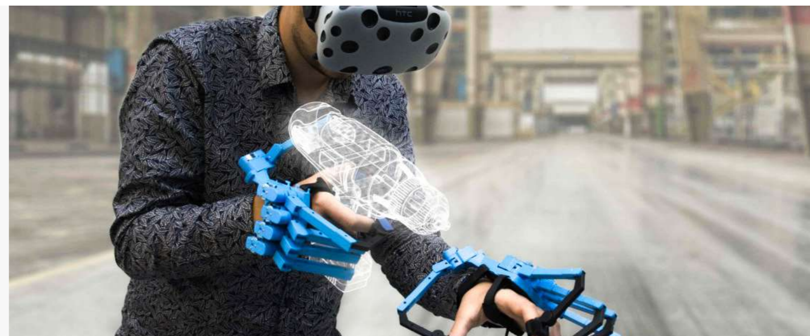
Figure 15 The SenseGlove being used for virtual training
