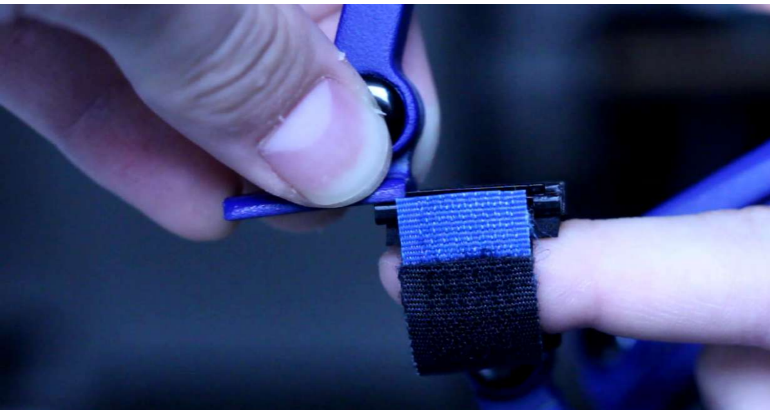
Figure 35 The swappable thimble integrated in the prototype
