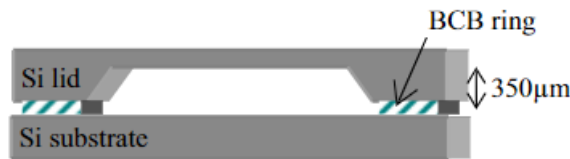
Figure 2.10: Structure of adhesive bonded test vehicle[29]
