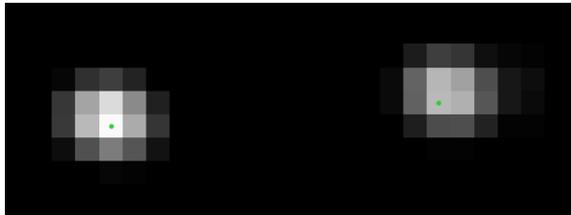
Figure 4.14: Initial peak location with integer pixel accuracy.
