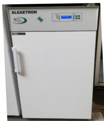
Figure 7: Incubator (Model: AlgaeTron AG 130-ECO)
