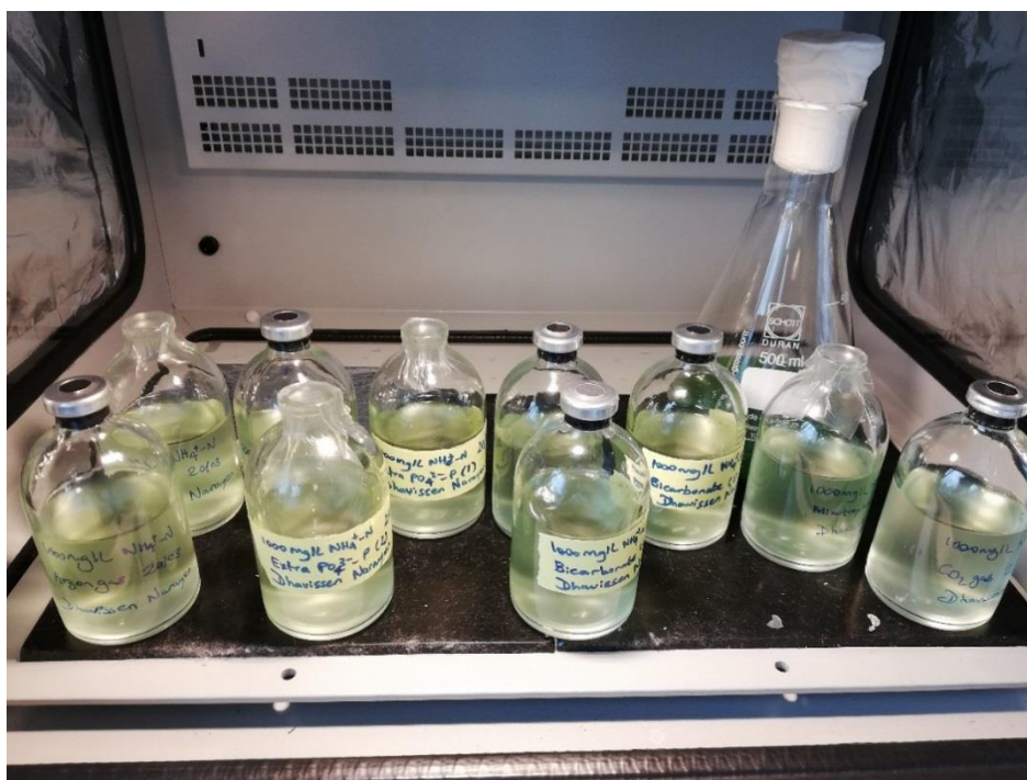
Figure 10: Cultivation of G. sulphuraria with different phosphate concentration and with bicarbonate and carbon dioxide supplementation in 100 mL serum bottles
