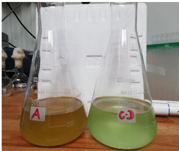
Figure 22: No growth of G. sulphuraria for the first time growth on 100% real RO concentrate having an iron concentration = 15.0 mg/L (left) and G. sulphuraria culture grown on synthetic RO concentrate (right) (Mixotrophic metabolism, conc. of \text{NH}_4^+ on day 0 = 200 mg \text{NH}_4^+ -N/L, C:N ratio on day 0 = 5:1, N:P ratio on day 0 = 37:1, pH = 2, temperature = 35 °C, light intensity of 80 \mu\text{mol photons m}^{-2} \text{s}^{-1} , light cycle of 14:10, shaker at 145 rpm).
