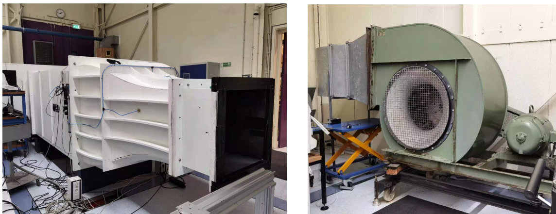
Figure 5.1: The contraction and test section (left) and the external ventilation system of the W-Tunnel, reproduced from [57]
