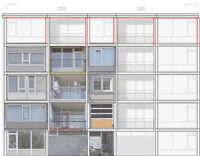
Figure 1.3.7. Concrete frame in Camera Obscuradreef filled with different elements
