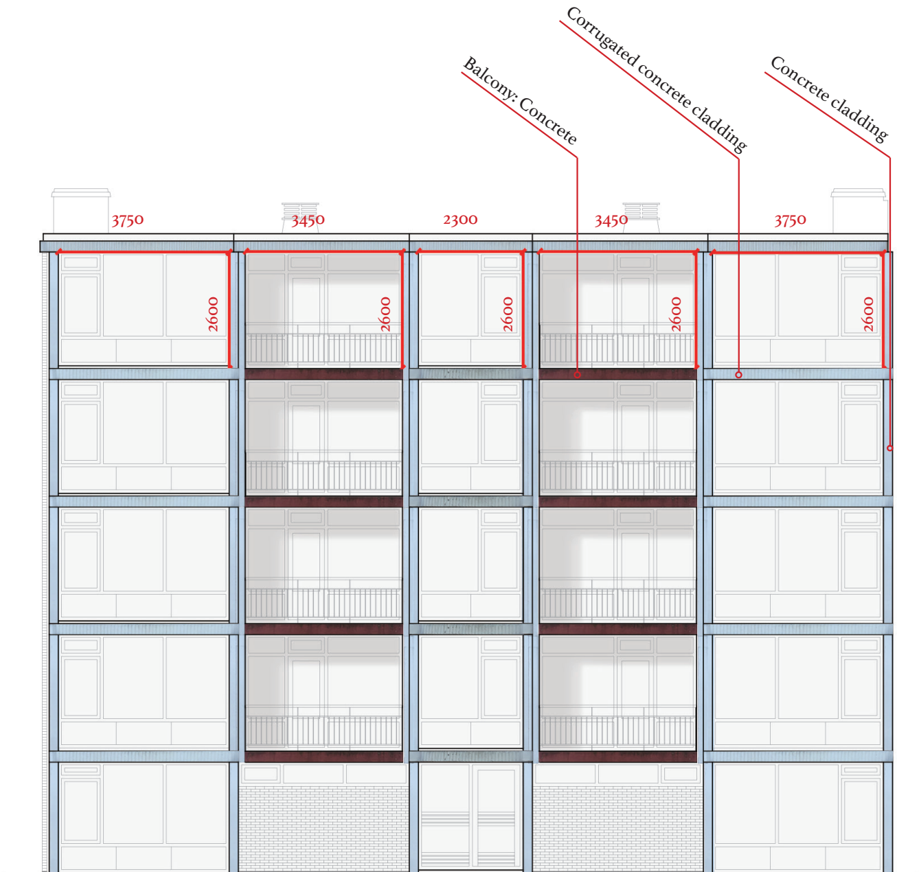
Figure 1.3.3 Overview of Concrete Frame in one portiek
