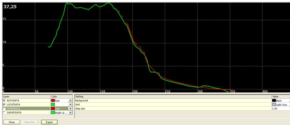
Figure 8.15: The profile of the beach measured by ALS Harrier56 system in April 2008 (green line) and by L-MMS StreetMapper system in November 2008 (red line) [Rijkswaterstaat, 2009].
