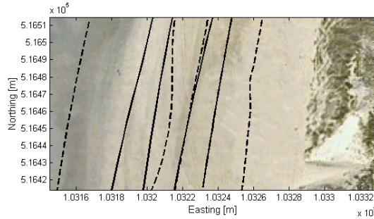
Figure 6.8: The digital photo of the test area [GoogleMaps]. The black dashed lines mark the trajectories driven downward i.e. from the north to the south and the solid lines mark the trajectories driven in the opposite direction.
