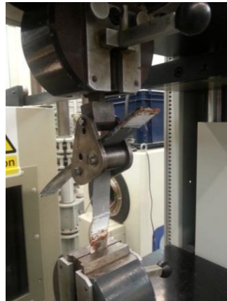
Figure 2: Floating roller peel test set up
