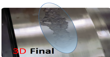
Figure 2.10: Final Spalling on the raceway surface[9]
