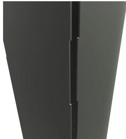
Figure 79: sheets fit into each other using 'puzzle pieces'
