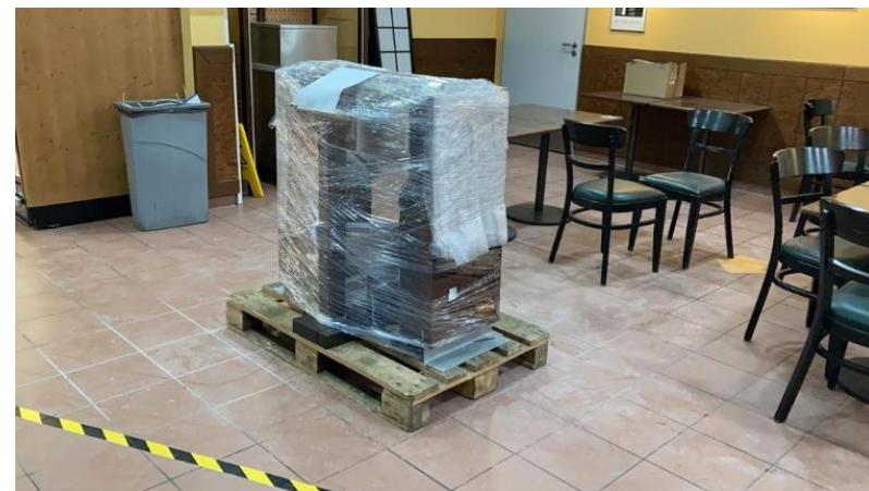
Figure 25: disassembled kiosk mounted to EUR pallet for transport
