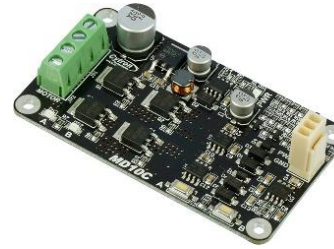
Figure 56: 2-way DC motor controller
