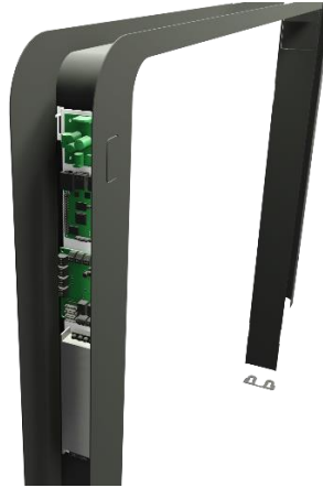
Figure 81: hardware plate neatly placed in frame
