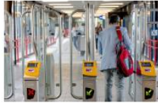
NS Stations 2 way gates, with QR code scanner and NFC reader 2 variations, one high and one low signage LEDs implemented, screen inside
