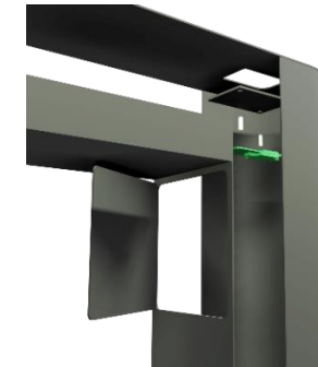
Figure 87: small door to reach the NFC reader
