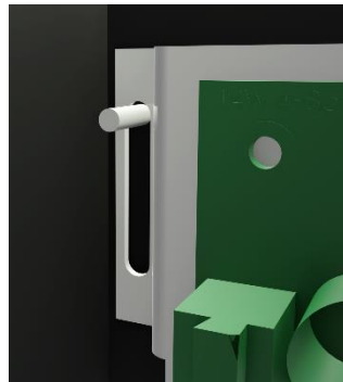
Figure 83: plate is screwed tight on welded threaded studs
