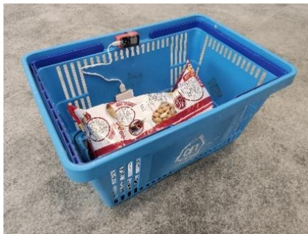
Figure 67: basket with BLE beacon attached
