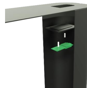
Figure 86: NFC reader in back pillar
