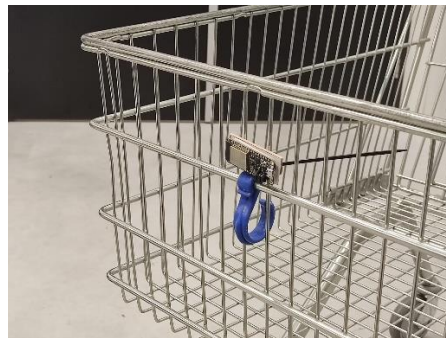
Figure 68: cart with BLE beacon attached
