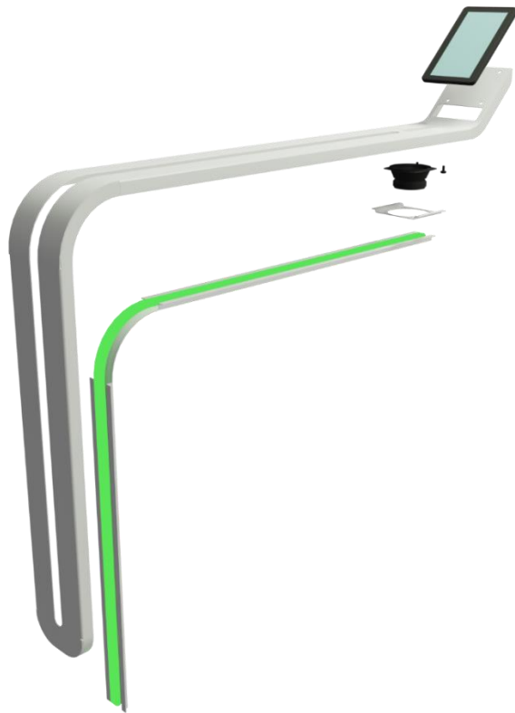
Figure 88: the cover housing the LED, speaker and screen
