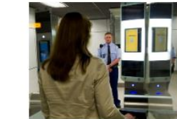
Schiphol Passport control with automatic face recognition Moving camera + lighting, specific spot for user to stand on
