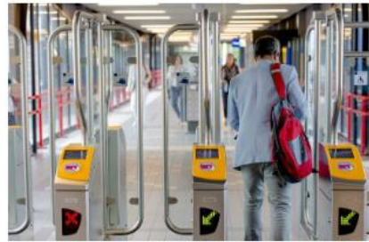
NS Stations 2 way gates, with QR code scanner and NFC reader 2 variations, one high and one low signage LEDs implemented, screen inside
