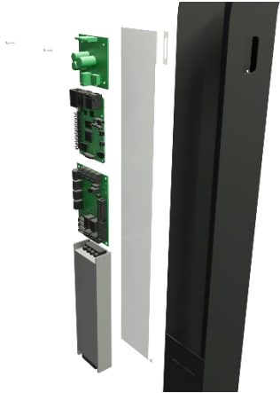
Figure 80: from top to bottom: soundboard, PanIO, Raspberry Pi, power supply
