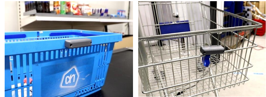
Figure 97: attaching the BLE beacon to a basket and cart
