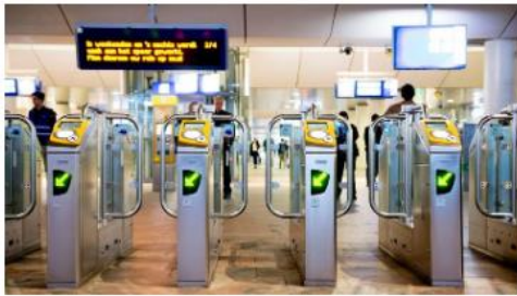
NS Stations 2 way gates, with QR code scanner and NFC reader 2 variations, one high and one low signage LEDs implemented, screen inside
