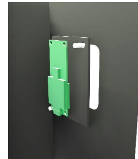
Figure 85: NFC reader in front pillar
