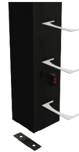
Figure 84: welded-in plates help distribute any impact forces
