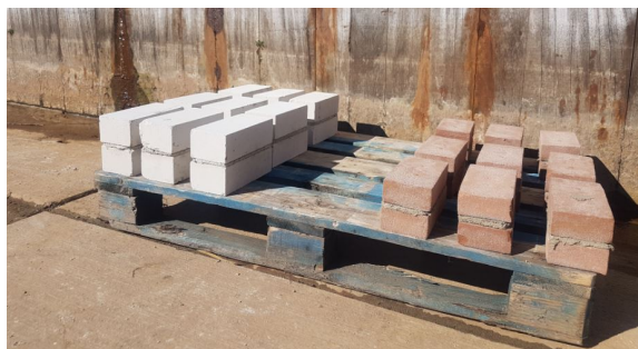
Figure 4.6: The couplets were left to harden next to the wall for the same duration.
