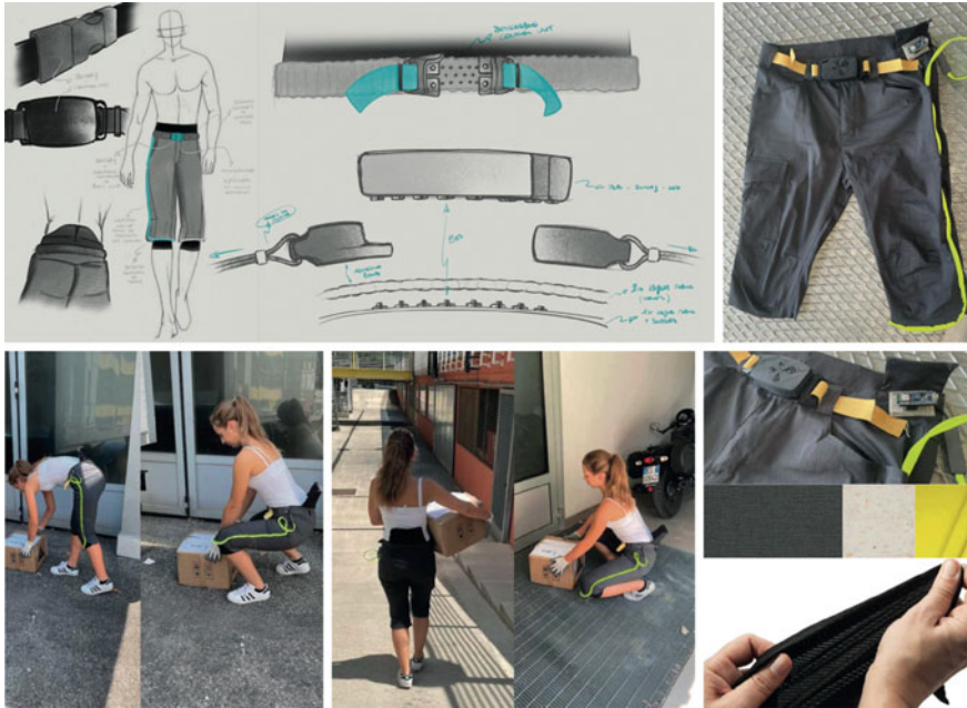
Fig. 16 Visualizations and prototype of SENSE-E WORKPANTS: tech-wear for repetitive strain injuries prevention. By Alice Ballestra, Ludovica Bonaldo, Francesco Carlucci, Hanna Selim
