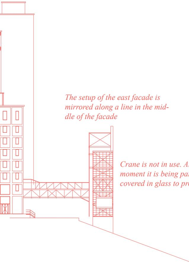
*The setup of the east facade is mirrored along a line in the middle of the facade*
